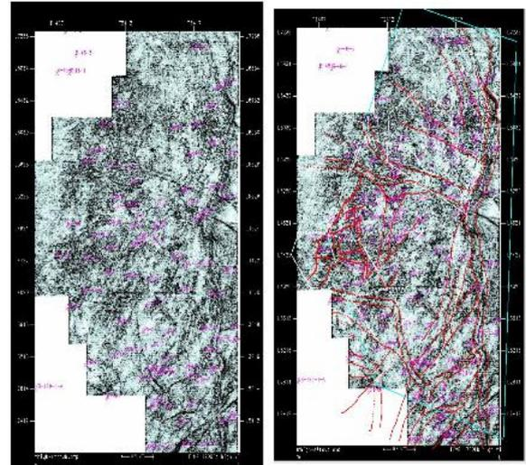
Figure 6: Structure cube slice @ 1700ms showing fault trends at Basement level
