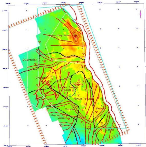
Figure 2: Structure map on top of Basement depicting different fault sets
