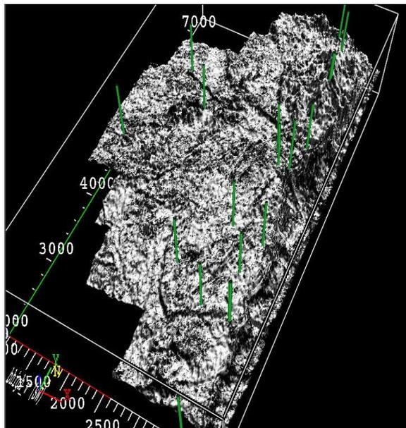
Figure 5: Structure cube attribute map on top of Basement depicting the Fault pattern.
