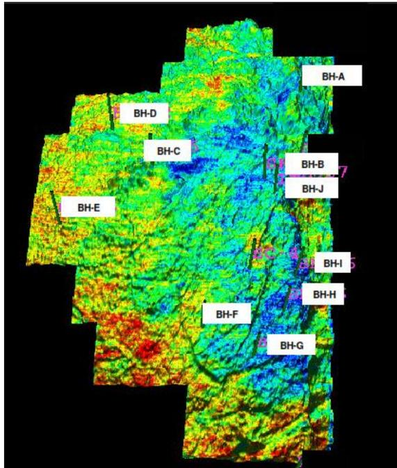
Figure 4: RMS Amplitude map of a 20msec window below Basement top depicting the fault pattern
