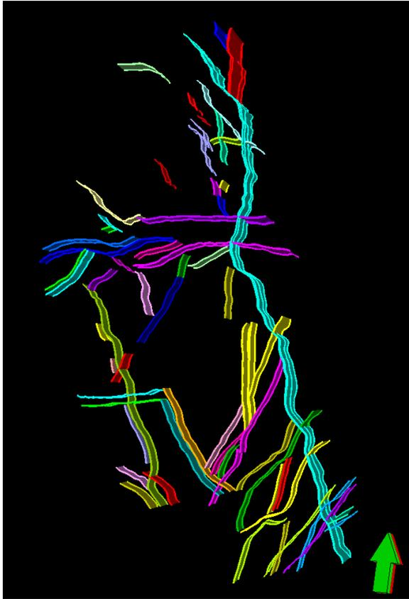
Figure.8: Major Fault sets at Basement top: Mumbai High field. Note the presence of dilatational jogs, lateral ramps and transfer faults
