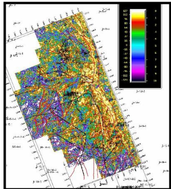
Figure 7: Amplitude variance Cube extract of 0 to 20 msec window below Basement top indicating probable development of fracture porosity along major fault zones.
