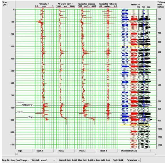
Fig 9: PP synthetic seismogram of Well X.
