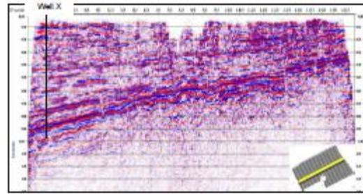
Fig 7: PSTM stack along the well X (Vertical comp.)
