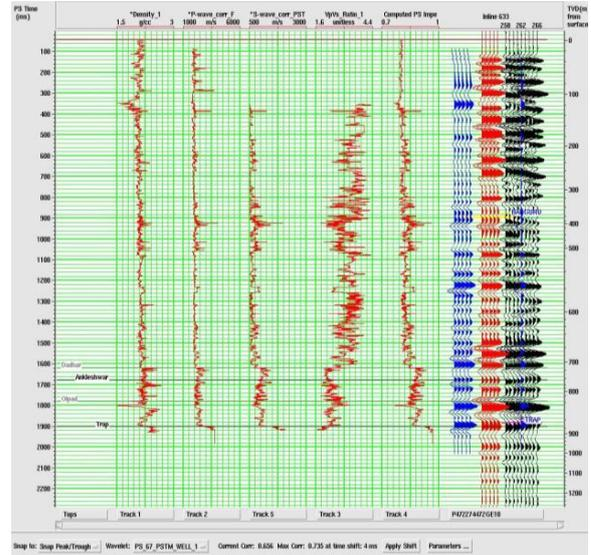
Fig 10: PS synthetic seismogram of Well X
