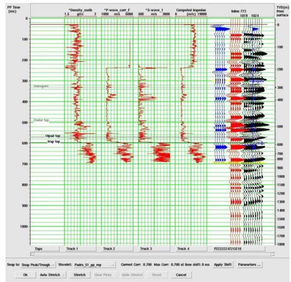
Fig 11: PP synthetic seismogram of Well Y.
