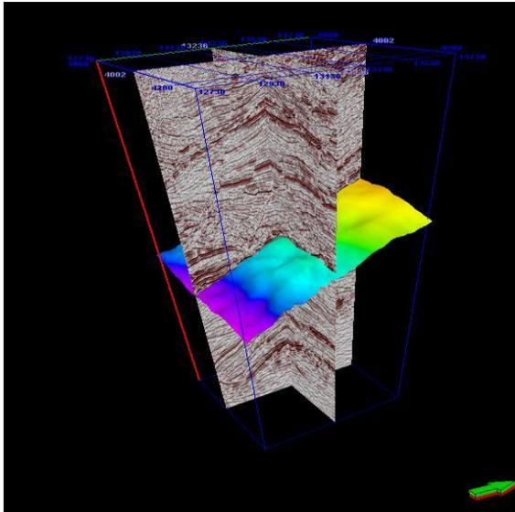
Figure 4: Sub surface with inline and crossline seismic sections.
