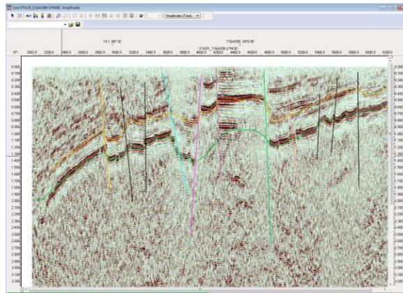
Figure 1: A interpreted seismic profile in 2 dimension showing marking of faults and horizons of interest
