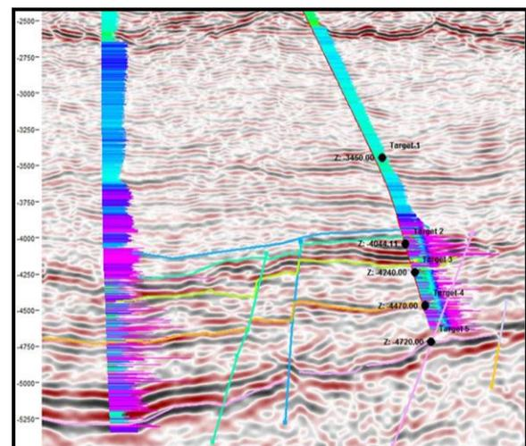
Figure 3: Section showing seismic to well tie and well to well tie
