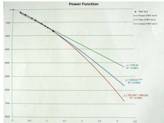
Figure 2: T-D plot to convert Time Domain to Depth Domain
