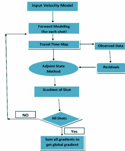
Figure 1: Flowchart for the solution of Eikonal and adjoint state equations
