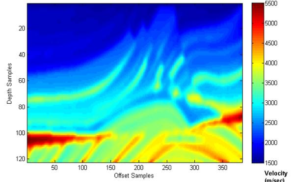
Figure 4: Smooth velocity model for adjoint state solution.
