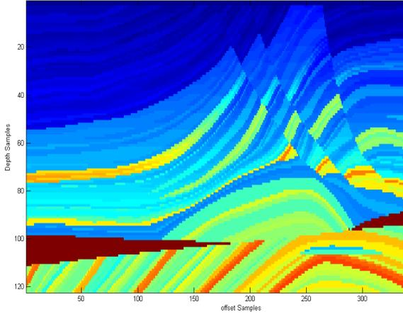
Figure 2: Marmousi velocity model
