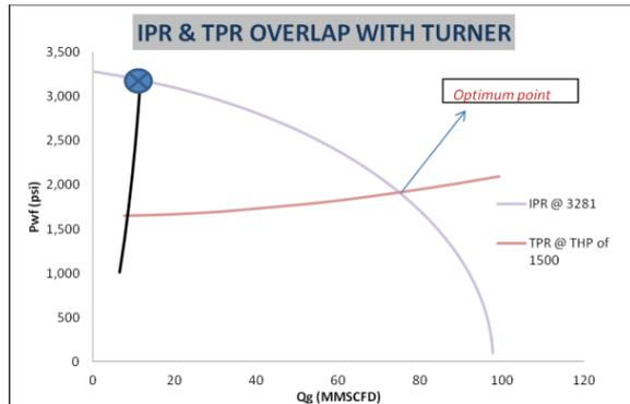
From this graph, we interpret that as long as the optimum point of the reservoir is on the right side of overlap point of IPR and Turner liquid loading does not occur.
