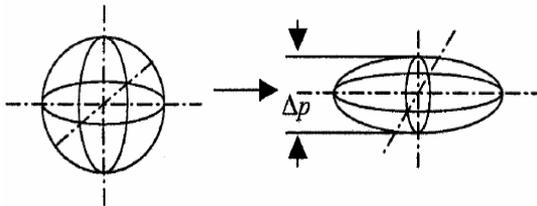
Spherical liquid droplets have a smaller efficient area and need a higher terminal velocity and critical rate to lift them to the surface. However, flat-shaped droplets have a more efficient area and are easier to be carried to the wellhead.
