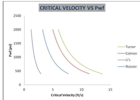
One can notice that Turner model gives the most conservative value of critical velocity of all the methods for any value of pressure. The Turner model is most widely used and accepted in oil and gas industries and moreover all the theories are based on the Turners model.
