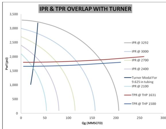
In this case, the TPR at THP of 1500 intersects with the IPR on the left hand side of intersection of IPR and Turner. This represents that at that pressure of well, liquid loading occurs.
