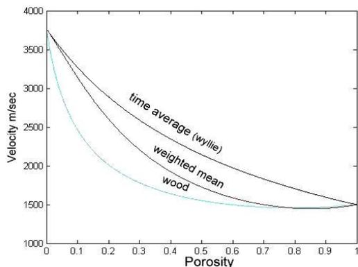
Figure 2: Graph showing the P-wave velocity trends at different porosity values obtained for the Wood's model, Wyllie's time average equation and the three phase weighted equations (W=1.2)
