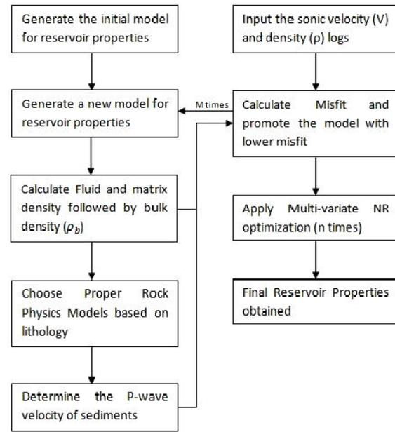
Figure 1: Flowchart demonstrating the workflow for the transformation from acoustic and density properties to reservoir properties based on rock physics modeling and multi-variate Newton Raphson inversion
