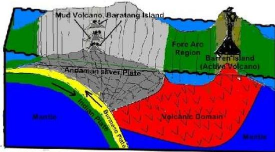
Figure 3: Accretionary prism showing avenues of fluid escape forming mud volcanoes due to seismic pumping.
