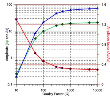
Figure 2: Change in P- and S-wave amplitudes with respect to attenuation (inverse of Q) are plotted in green and blue colors, respectively. Amplitude factor is the ratio of P- and S-wave amplitudes and is shown red color.
