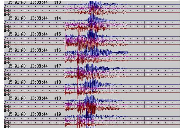
Figure 1: Example of microseismic data for a number of multicomponent geophones. Vertical component is in blue color and two horizontal components are in purple and red colors.
