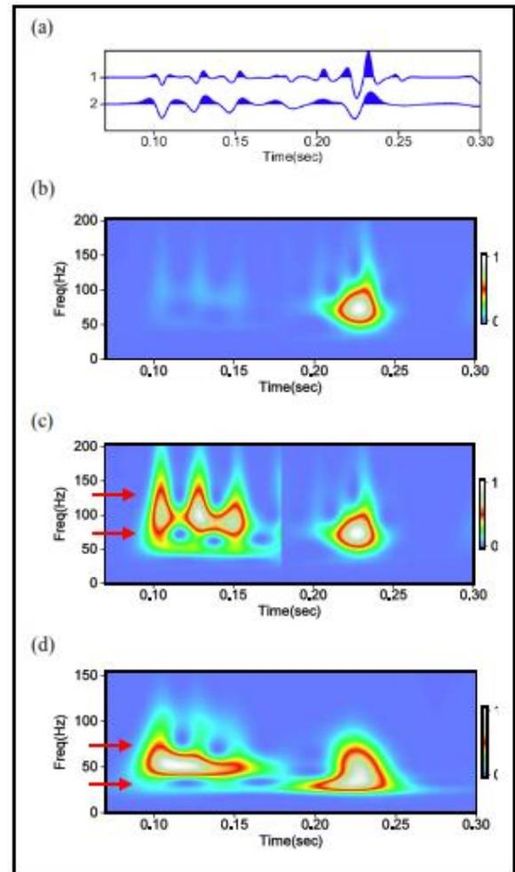
Figure 3: (a) Synthetic seismograms for  $Q = 100$  (trace 1) and  $Q = 10$  (trace 2) (b) Spectral decomposition of trace 1 and partly enhanced amplitudes between 0 and 0.18 sec (c). (d) spectral decomposition of trace 2.
