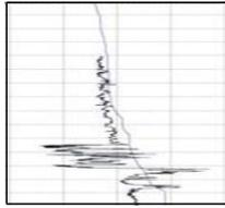
Figure 2: P-velocity wireline log (black) and seismic interval velocity log (blue).
