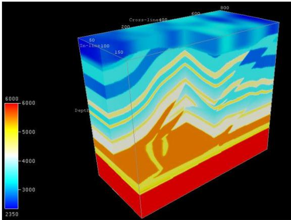
Figure 3: A schematic of the SEG/EAGE overthrust model. Colour bar represents the p-wave seismic velocity is m/sec.
