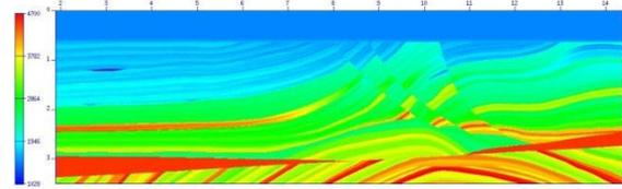
Figure 1: A schematic of Marmousi-II velocity model. The colour bar on left represents p-wave seismic velocities in m/sec.
