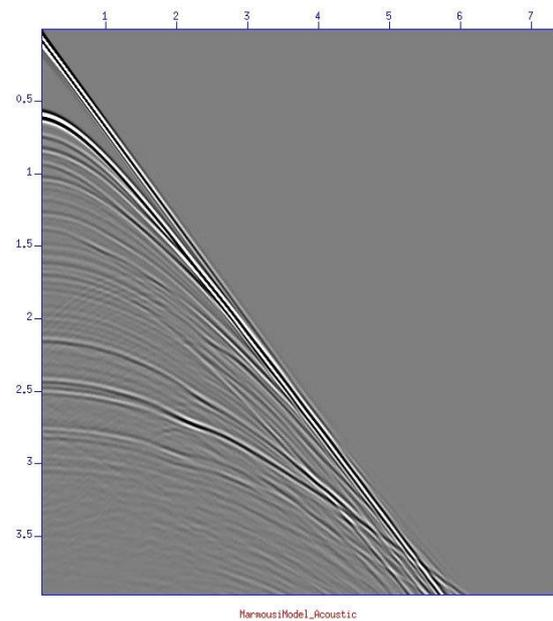
Figure 2: Synthetic seismograms obtained from 3D acoustic wave modeling algorithm for the Marmousi-II model.
