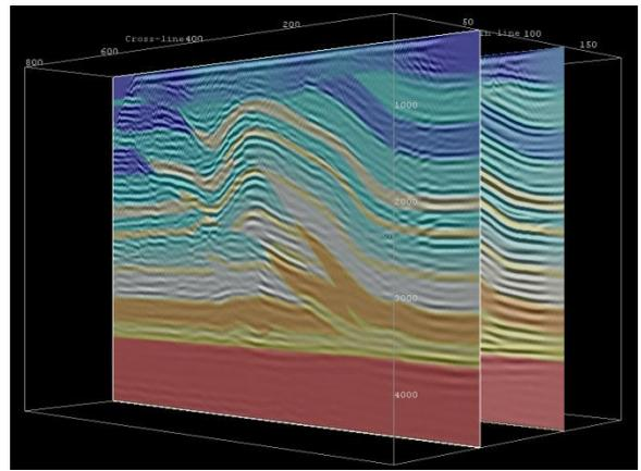
Figure 4: The seismic image obtained after 3D RTM of the overthrust model along two inlines. The velocity model is also superimposed on the migrated section.
