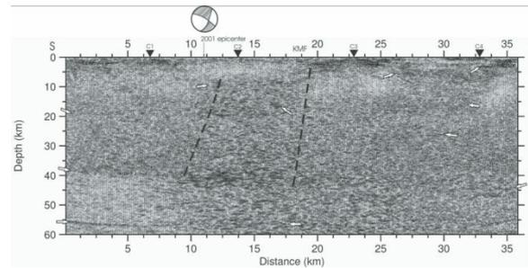
Pre-stack depth migrated section along a profile running across the 2001 epicentral region. Prominent reflection boundaries are represented by white arrows. Hypocenter of the Bhuj earthquake along with the focal mechanism as viewed on a vertical cross section is also shown. Moho is at a depth of 38-45km. (Sarkar et al, 2007).
