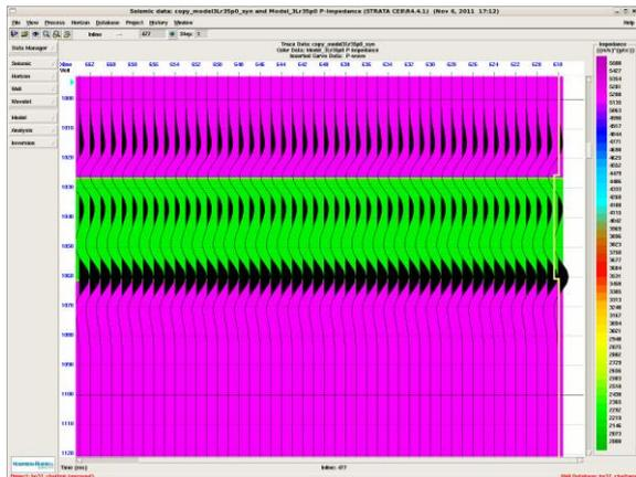
Fig. 2 Three layered initial model with ricker wavelet (after Anstey N. A., 1978)
