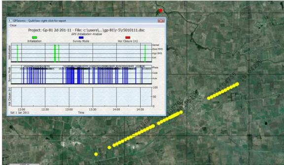
Fig. 3 (RTK initialization analysis)
