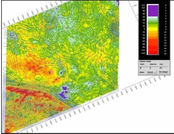
Fig.10: Computed porosity at Upper Pay level (Red to yellow colour shows higher porosity while green to blue represents lower porosity)
