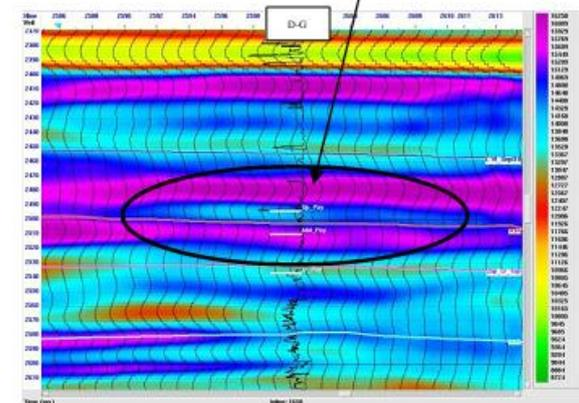
Fig.7: Acoustic Impedance section through well D-G. High AI values shows tight lime stone.
