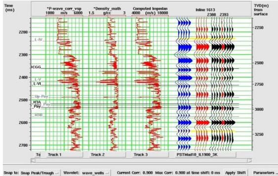
Fig.5: Calibration of seismic data with well logs & generation of synthetic trace. Correlation is 90%
