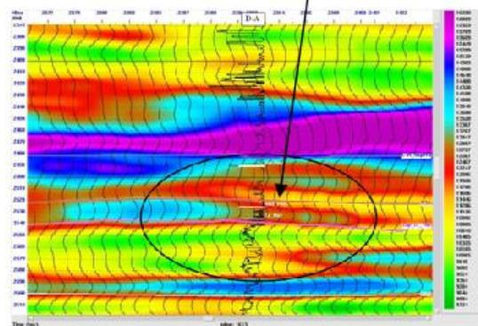
Fig.6: Acoustic Impedance section through well D-A. Three reservoir layers are well resolved
