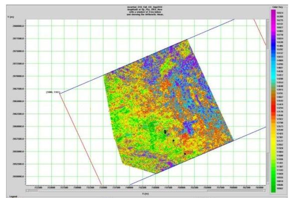
Fig.8: Distribution of acoustic impedance for Upper Pay. Violet to blue patches indicates high AI values and tight lime stone.
