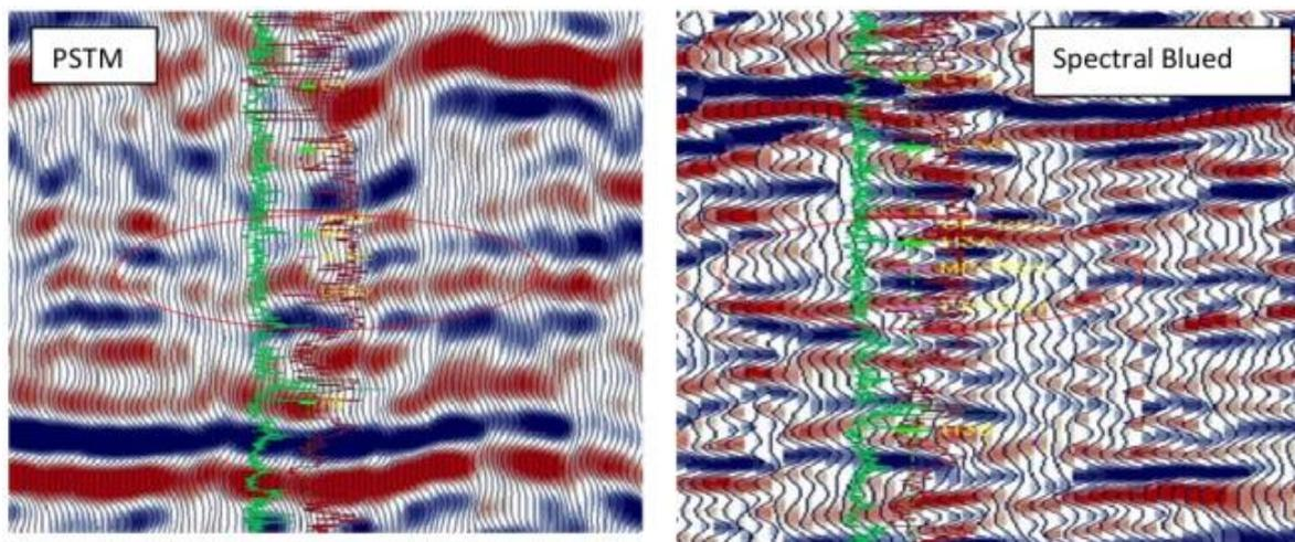
Fig.4: Zoomed sections of In Line 1613. Comparison for frequency enhancement after applying Spectral Blueing
