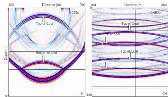
Figure 3: Wave-field propagation at two different time steps (0.022s and 0.052s). The elastic wave-field showing both (up and down going waves); the top of the coal layer exhibits the reverse polarity. (a) is a snapshot of wave-field at 0.22 s for flat layer model; (b) is representing the wave- field propagation at 0.52 s.
