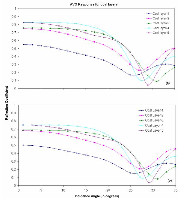
Figure 6: Comparison of AVO curves produced for a multi-layered anisotropic model. The reflection coefficient is calculated for all the five coal layers. The AVO response is modelled up to 35° (a) In this case the source receiver spacing is 50 m. (b) In this case the source receiver spacing is 10 m.
