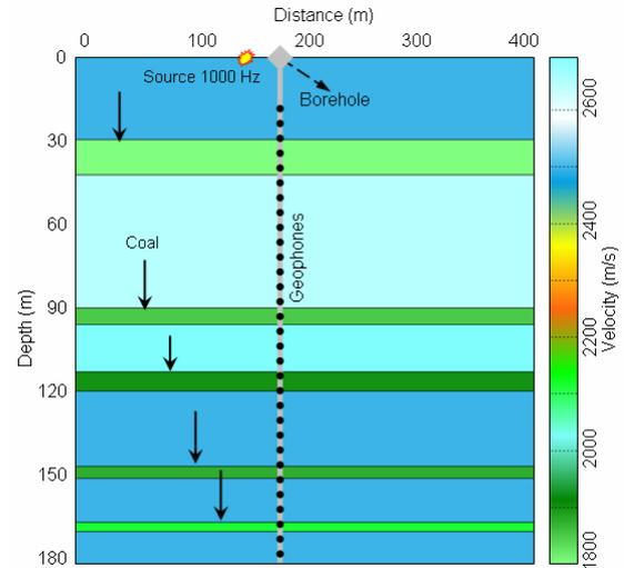
Figure 1: Flat stratigraphic layer model for vertical moving source and vertical receivers. Black arrows (solid line) are showing coal layers. Source-receiver distance is 10 m.
