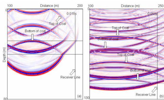
Figure 5: Wave-field propagation at two different time steps (0.018s and 0.050s), (a) is a snapshot of wave-field propagation at 0.18s; (b) is representing the wave-field propagation at 0.50 s.
