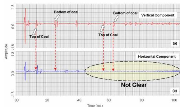
Figure 4: Simulated seismic response two components (flat layer model). The source is positioned at 1 metre depth and receiver positioned at 5 m depth with 50 m source receiver spacing. (a) Vertical component response up to 100 ms; (b) shows the horizontal component response up to 100 ms.
