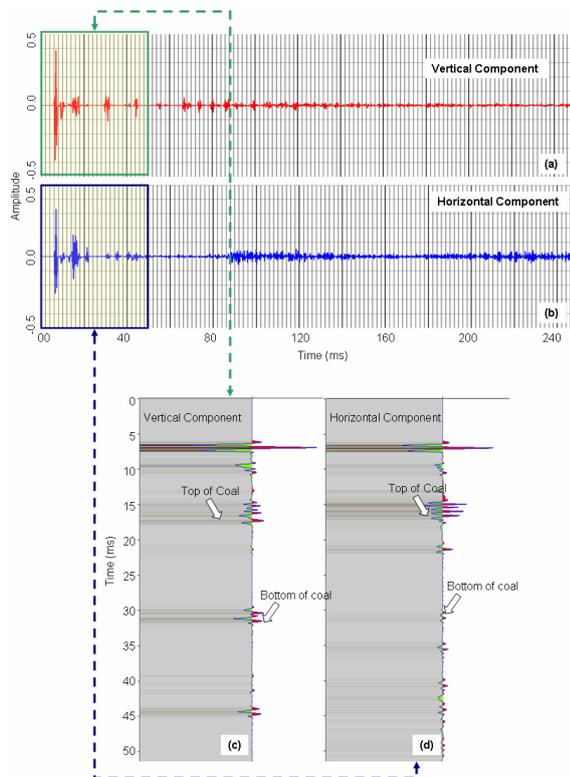
Figure 2: Single receiver response for two components (flat layer model Fig. 1). The source is positioned at 25 meter depth (a) Represents the vertical component response up to 250 ms. (b) shows the horizontal component response up to 250 ms. (c) Represents the enlarged green box area from 'a' up to 50 ms. (d) shows the enlarged blue box area from 'b' up to 50 ms.
