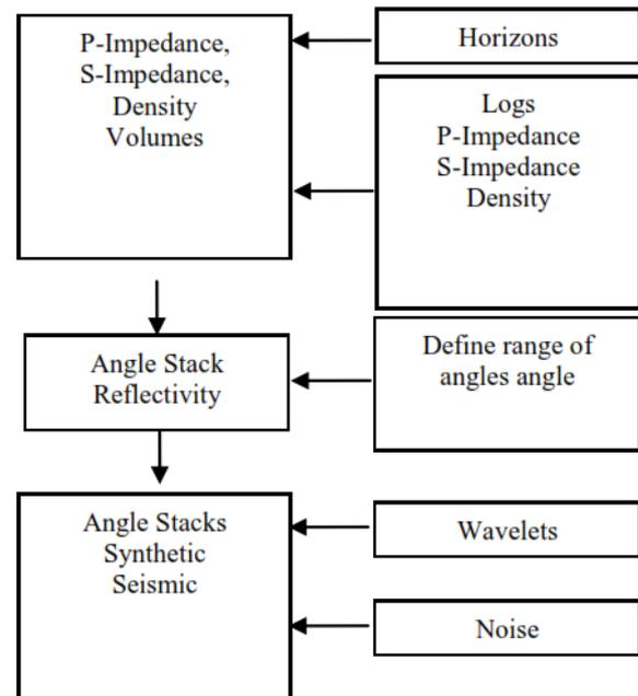
Figure 1 Forward Modeling (Workflow)
