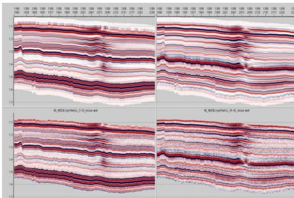
Figure 2 Synthetic data created through Forward Modeling without and with Noise
