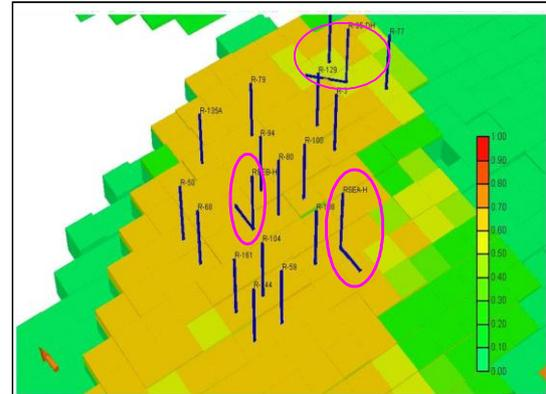
Figure-6: Placement of Horizontal well & SRDH
