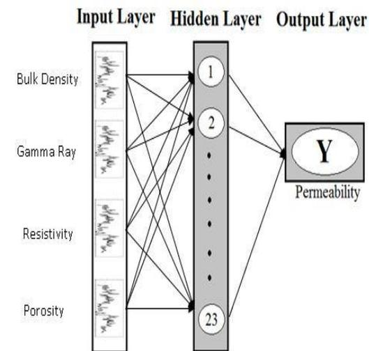
Figure 2: Network architecture of BPNN showing input layer, hidden layer, and output layer, and connecting weights. back propagation neural network (BPNN) has been used for permeability estimation.
