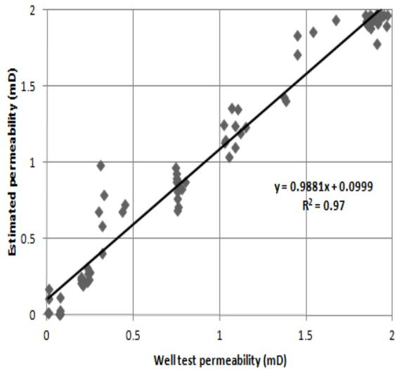
Figure 5: Best fit relation between well test coal-bed permeability and network predicted coal-bed permeability for well A.
