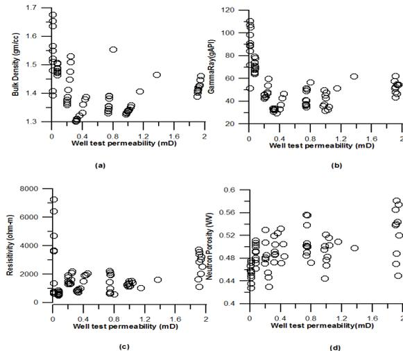
Figure 1: Displays scattered cross-plots of (a) Bulk density, (b) Gamma ray, (c) Resistivity analysis. ANN is a computer model and (d) Neutron porosity with well test permeability for coal seams of wells of the Damodar valley coalfield, India.
