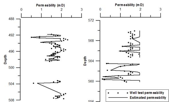
Figure 7: Permeability vs. depth profile of coal seams of well B.
