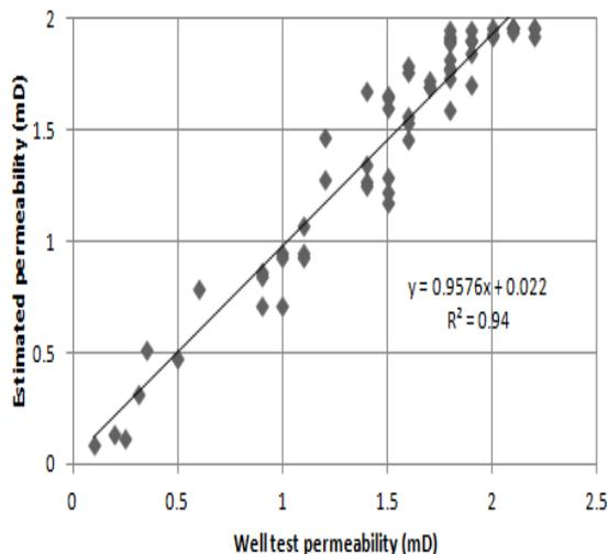
Figure 6: Best fit relation between well test coal-bed permeability and network predicted coal-bed permeability for well B.
