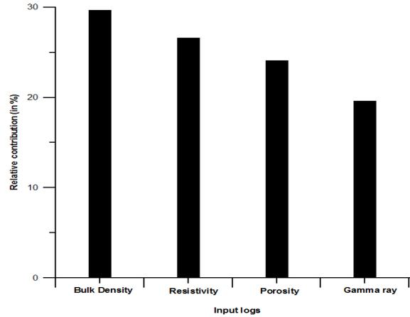
Figure 4: Contribution of input logs to permeability estimation.
