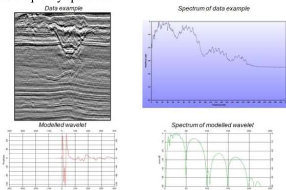
Figure 8. Data example together with wavelet and spectra, for hydrophone-only data. Source and receiver ghosts, source signature, and earth's absorption are all present. The frequency range shown in the amplitude spectra is 0-250Hz, vertical axis represents amplitude in dB, with zero at the top, and -10dB increments. The bottom left shows the extent of the wavelet, with the vertical axis representing amplitude, and the horizontal axis time, with 100ms increments.
