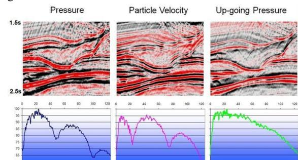
Figure 3. Hydrophone, Velocity sensor, and resulting amplitude spectra for dual-sensor streamer at 15m tow depth. (Frequency range is 0-120Hz.)
