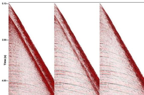
Figure 7. Shot record from depth & time distributed source. Left: as recorded, Centre: After de-ghosting Right: after de-ghosting and source separation.
