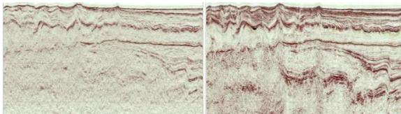
Figure 4. De-ghosted dual-sensor data from offshore Cyprus (right) shows improved resolution and penetration compared to conventional streamer data (left)
