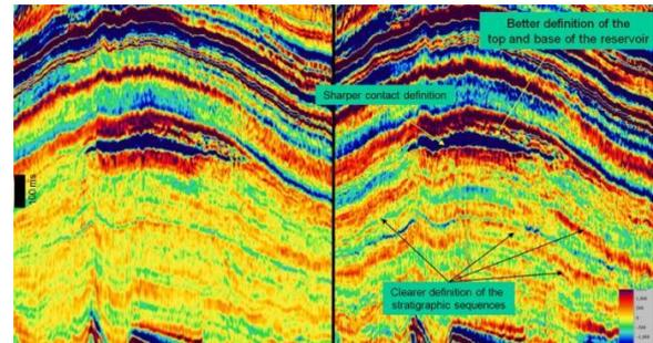
Figure 5. A relative inversion exercise over a large gas reservoir from the NWS Australia. Conventional streamer data (left), and de-ghosted dual-sensor data (right).
