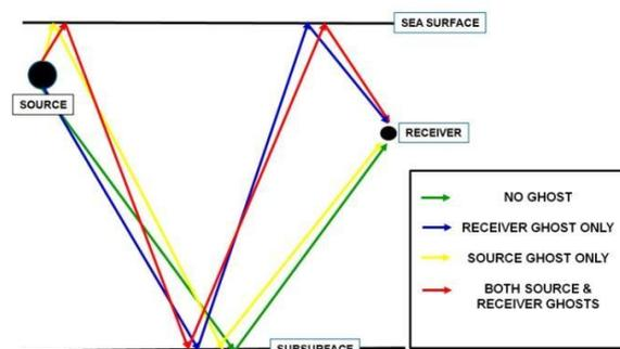
Figure 1. Raypaths showing source and receiver ghosts in towed marine seismic.
