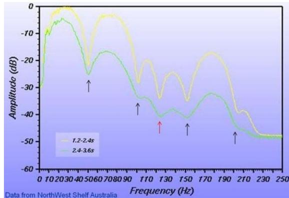
Figure 2. Receiver ghost notches (black arrows) and source notch (red) for streamer at 15m tow depth.
