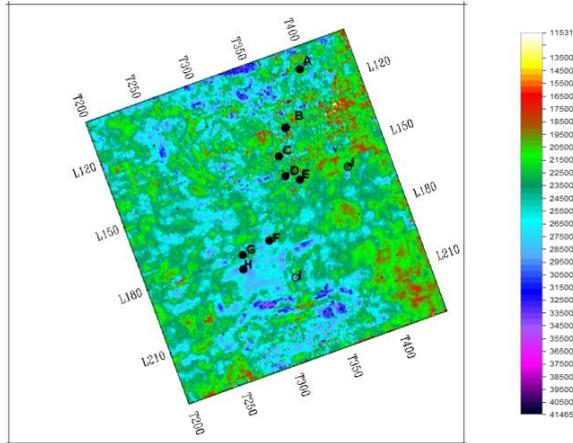
Fig 10. Amplitude Map of KIX sand (0 to 6ms from sand top)
