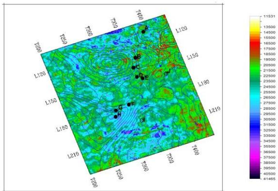
Fig 11. Amplitude Map of KIX sand (0 to 6ms) overlain by structure at KIX sand.
