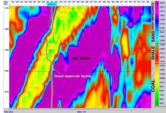
Fig 8. Impedance section through Well B overlain by GR log
