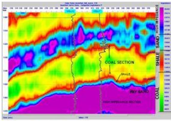
Fig 7. Impedance section through Well F overlain by Impedance log
