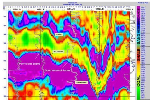
Fig 9A. . Impedance section through Wells G,F,E,B & A overlain by GR log
