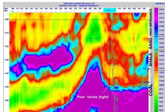
Fig 9A. . Impedance section through Well J overlain by Impedance log
