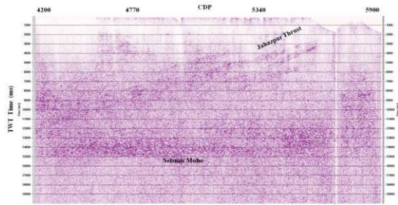
Fig.3 CMP Stack Section of Nagaur Jhalawar geotransect
