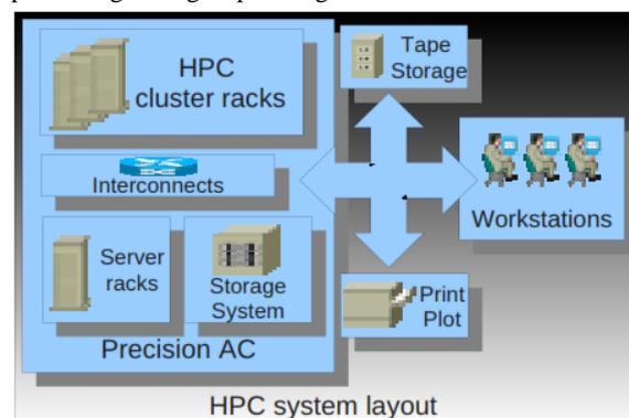
Figure 1: HPC technology building blocks.
