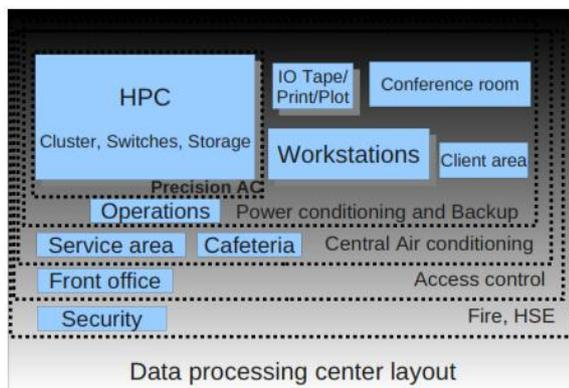
Figure 2: Data processing center layout
