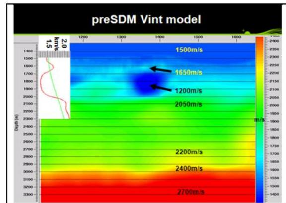
Figure 2: corresponding interval velocity profile used for the 3D preSDM. The inset in the upper left corner shows a velocity profile extracted through the geobody, clearly indicating the increase in velocity at the top of the body
