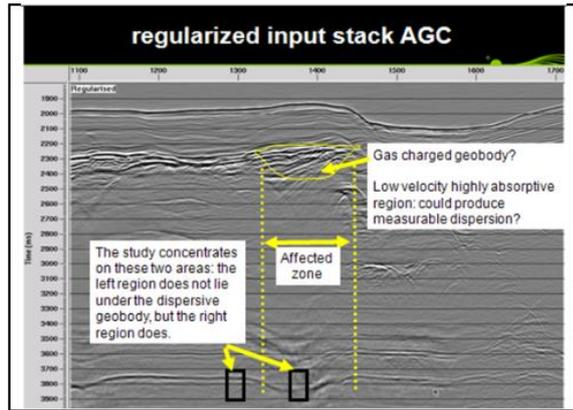
Figure 1: data in study area showing low velocity geobody and associated underlying pull-down and dimming
