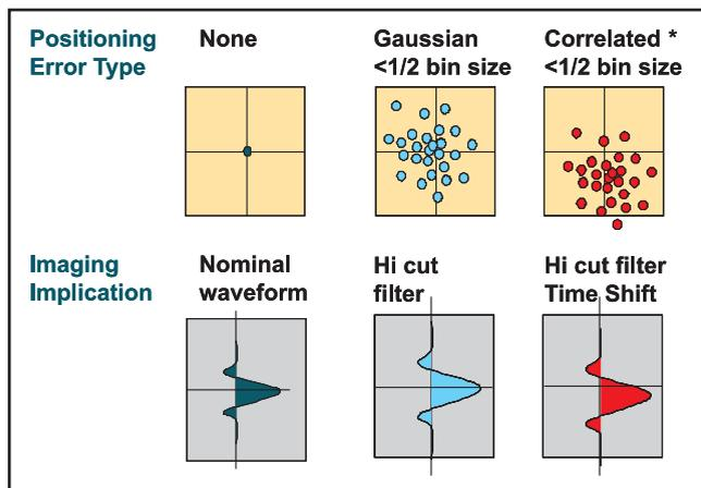
Fig-4. Illustration of impact of positioning errors on seismic wavelet.
