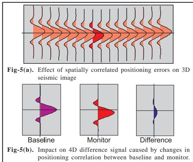
Fig-5(a). Effect of spatially correlated positioning errors on 3D seismic image
