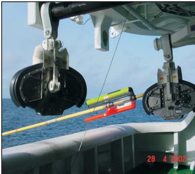
Fig-1. Integrated magnetic heading sensor and cable leveling device ("bird") mounted on towed streamer
