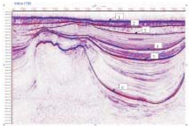
Fig. 3 : seismic section with salt structure
