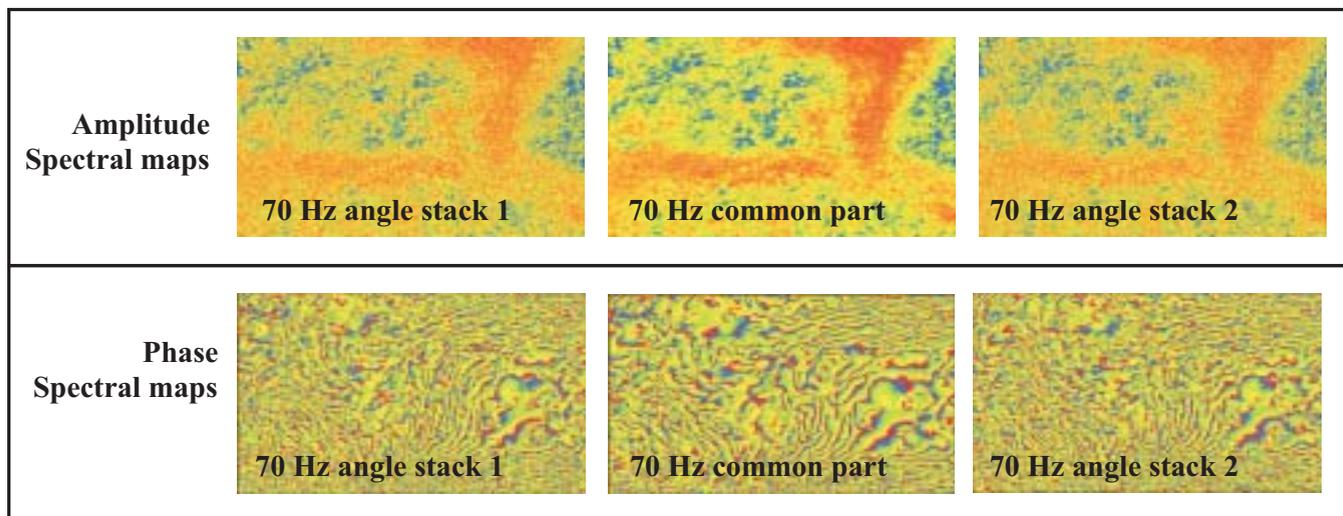
Fig. 2: High frequency recovery after a factorial co-kriging operator applied on phase and amplitude spectral maps. The frequencies of the common part, corresponding to an intermediate partial stack, are constructed from the coherent information.
