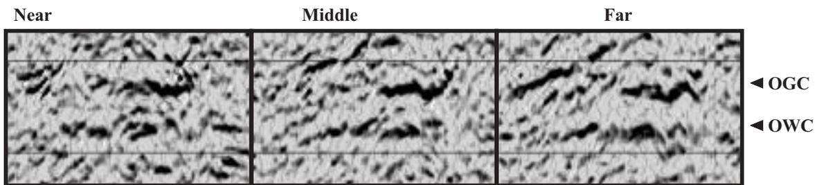
Fig. 5: High-resolution 4D signatures on different angle stacks. Near, Mid, Far
