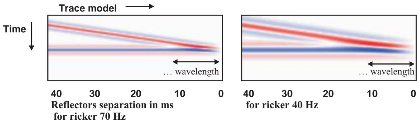
Fig. 1: The panels represent a 1D seismic difference model with a gradual decreasing distance/time between two reflectors (same reflection coefficient). The reflector separation varies from 40 to 0 msec with a step of 0.4 msec. The tuning effect is reduced for the high frequencies.
