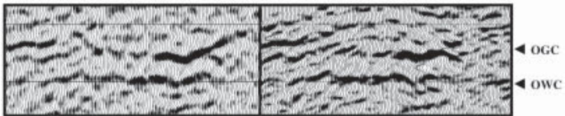
Fig. 4 : 4D signature before and after high frequency broadening. The resolution of the variation of the oil-water contact and the oil-gas contact are improved after the high frequency enhancement. Some lateral continuity ambiguities of the 4D signature can be clarified.
