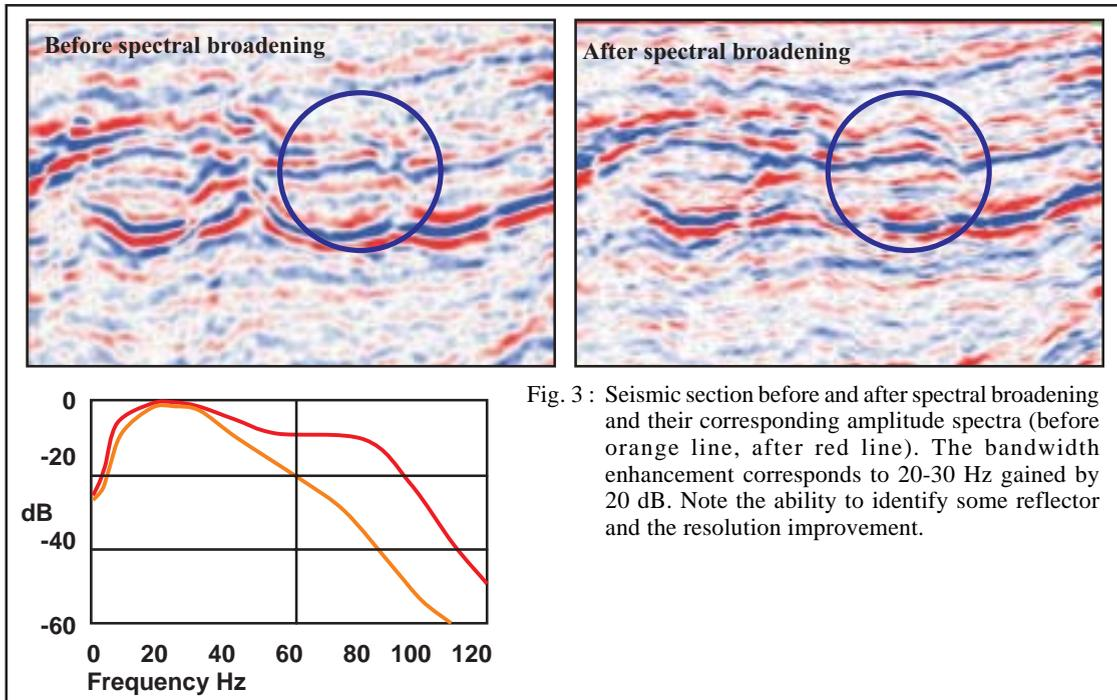
Fig. 3 : Seismic section before and after spectral broadening and their corresponding amplitude spectra (before orange line, after red line). The bandwidth enhancement corresponds to 20-30 Hz gained by 20 dB. Note the ability to identify some reflector and the resolution improvement.
