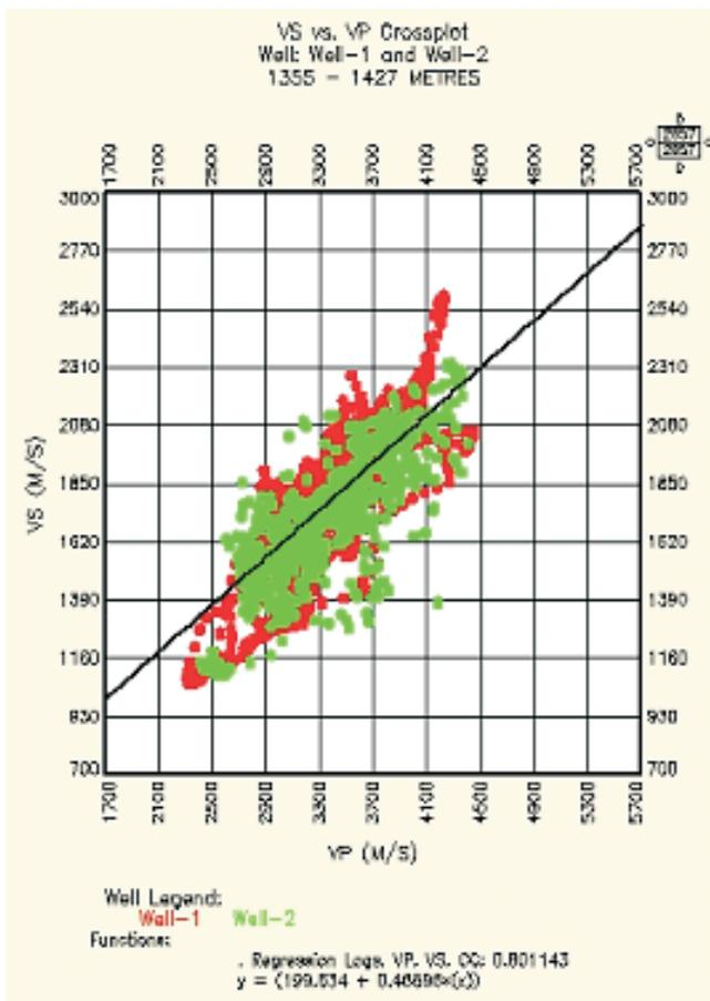
Fig.5 : Cross-plot between Vp and Vs
