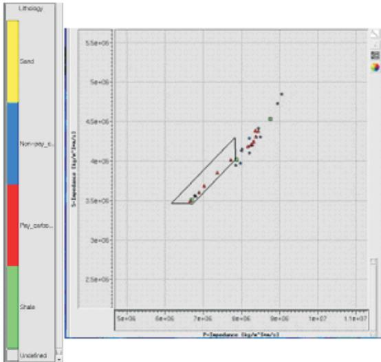
Fig.1 : Cross-plot between P-Impedance and S-impedance.
