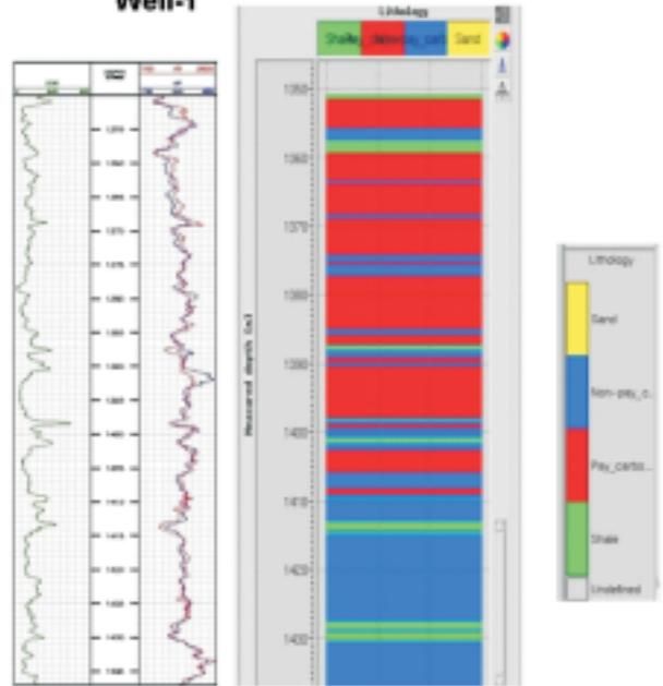
Fig.3: Dual Sonic, Gamma ray and Lithology of L-III reservoir of well-1
