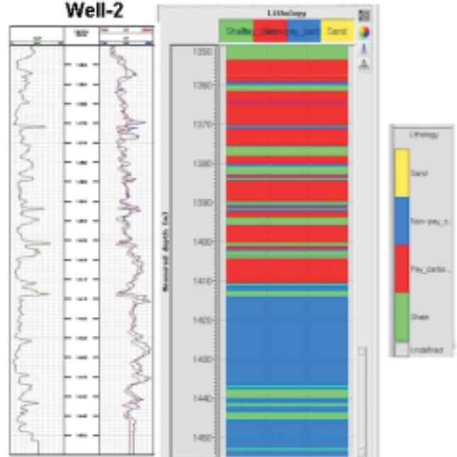
Fig.4: Dual sonic, Gamma ray and Lithology of L-III reservoir of Well-2
