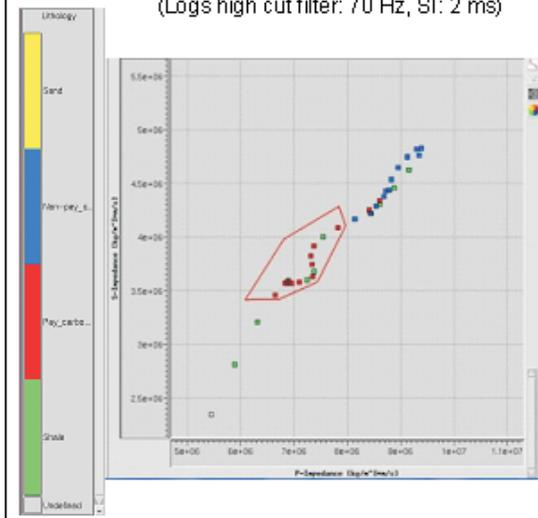
Fig.2 : Cross-plot between P-Impedance and S-impedance.
