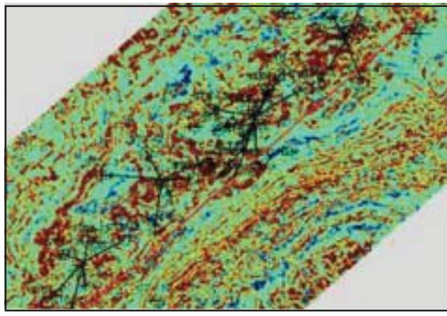
**Fig.8:** Number of zero crossings attribute analysis over the whole Zone II reservoir interval for the central part of the South Tapti Field, indicating the extent of shale interbedding within Zone II.
