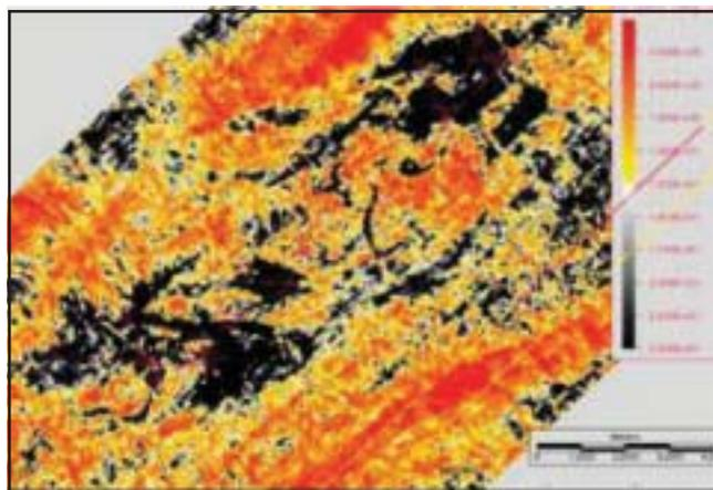
Fig. 3: Total energy extraction over the whole Zone II reservoir interval for the central part of the South Tapti Field, showing the maximum development of reservoir sand.
