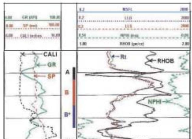
Fig. 1: Suite of Logs for lower sand-1 (LS-1) of Cambay Shale in Ankleshwar field
