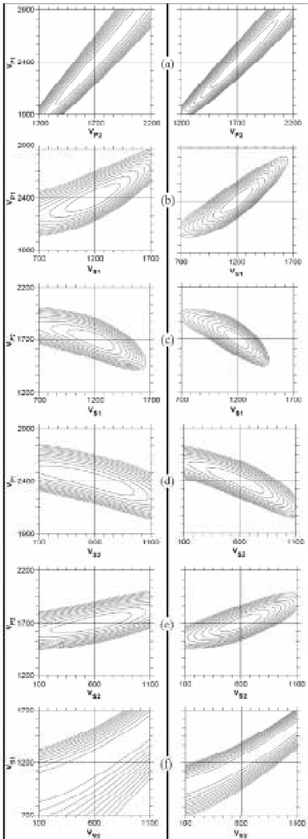
Fig. 4. Residual function mapping for AVA responses upto maximum angle of 30° (left panel) and 40° (right panel), investigating the linear dependence between (a)  $V_{p1}$  and  $V_{p2}$ , (b)  $V_{p1}$  and  $V_{s1}$ , (c)  $V_{p2}$  and  $V_{s1}$ , (d)  $V_{p1}$  and  $V_{s2}$  and (e)  $V_{p2}$  and  $V_{s2}$  and (f)  $V_{s1}$  and  $V_{s2}$  pairs. Crossing hair marks true values. Contour values range from 0.01 to 0.1 in steps of 0.01. Velocities are in m/s.
