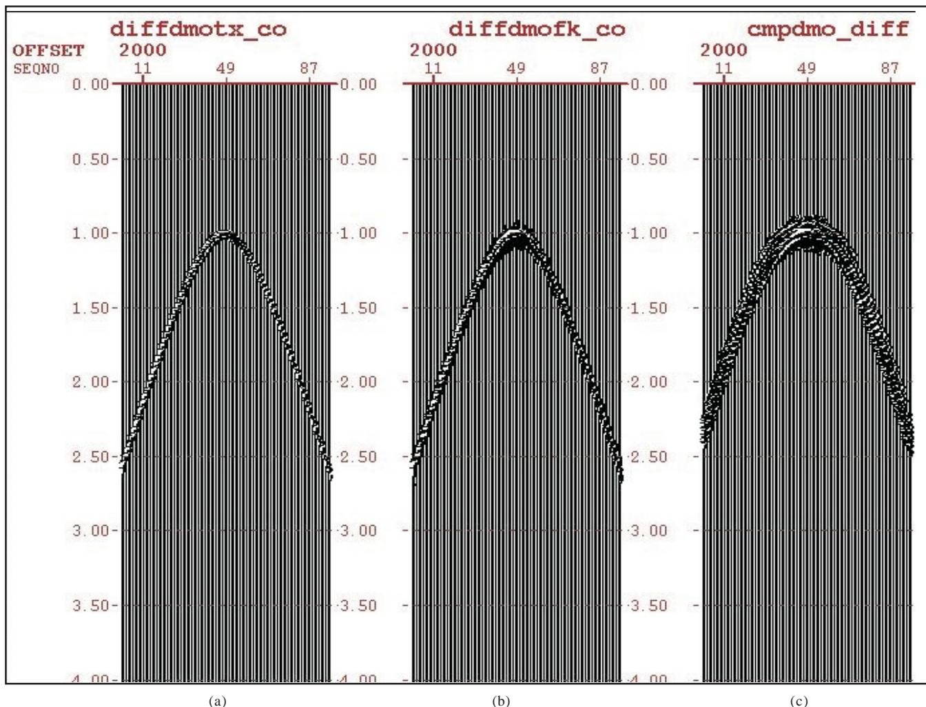
**Fig. 6.** Comparison of different DMO schemes applied to common offset section in fig. 5(a)
