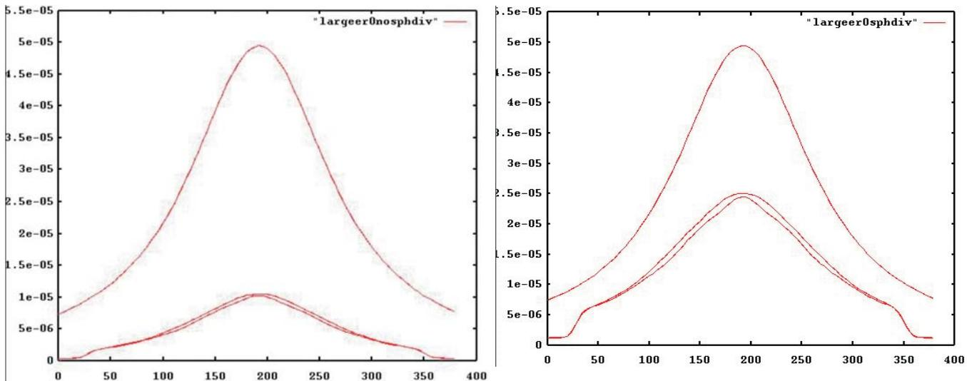
Fig. 9. A comparison of amplitudes obtained by f-k DMO of Hale and nonaliased t-x DMO.
