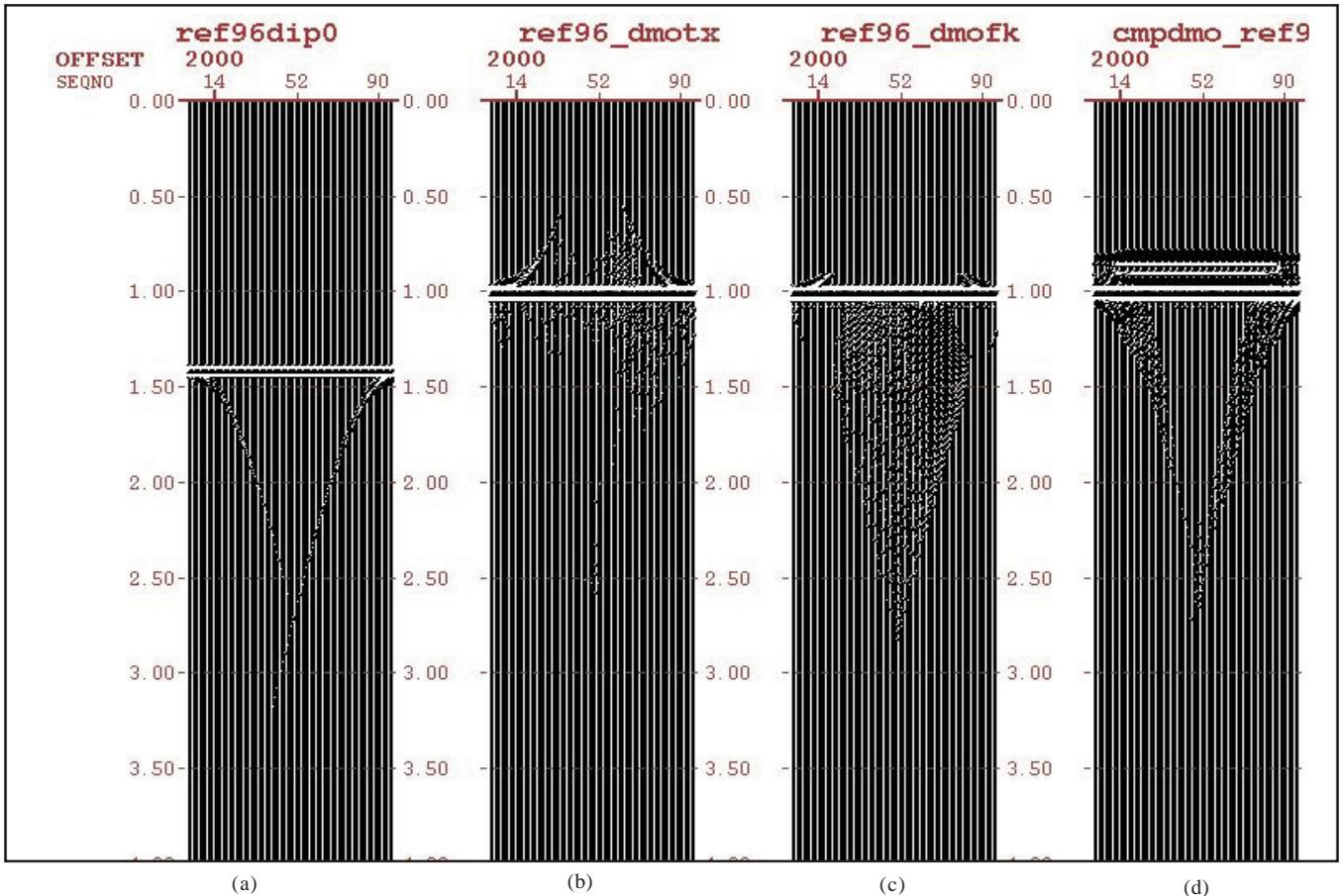
Fig. 8. Fig. 8a shows input common offset(2000m) data with a horizontal reflector. Fig. 8b shows the result obtained from nonaliased t-x dmo due to Hale. Fig. 8c shows the output of f-k dmo of (Notfors & Godfrey's version) of Hale's DMO whereas Fig. 8d shows the result obtained from t-x DMO of Deregowski & Rocca.
