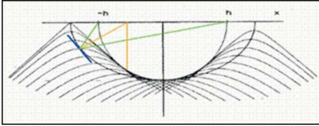
**Fig.2.** For a given source receiver pair, the travel time  $t_h$  is same for all points on the migration ellipse. Considering the migration ellipse as the reflector, construct a zero offset section. The outcome is the DMO impulse response. The zero offset point diffraction hyperbolae from all points on the migration ellipse, define the DMO impulse response.
