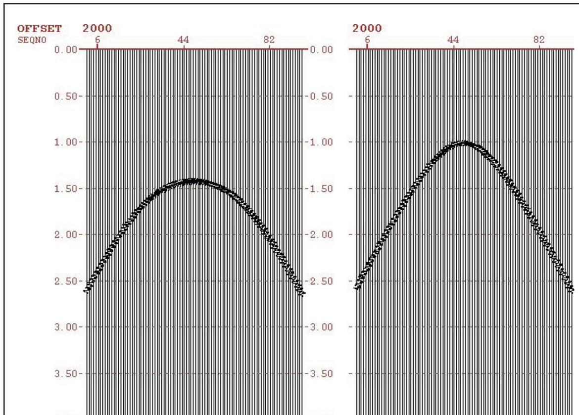
(a) Point diffractor: common offset(2000m)
