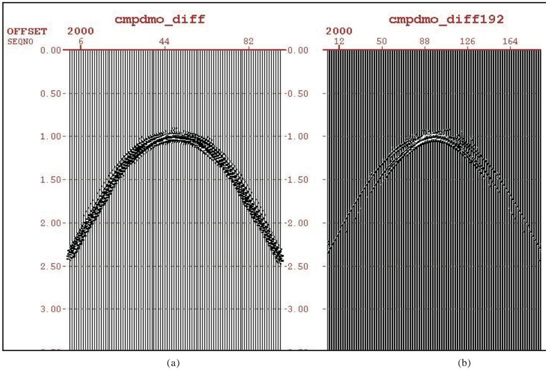
Fig. 7.(a) : Deregowski & Rocca's t-x DMO output with CMP interval equal to 50m. (b): with CMP interval 25m.
