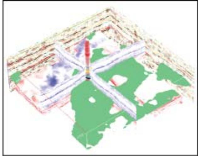
**Fig. 8:** Comparison of inversion input geo-cube, 1 of the 6 input angle-stack seismic cubes, and 2 resulting porosity cubes. The reservoir interval cube is built at flow unit scale of approximately 1 meter thickness.
