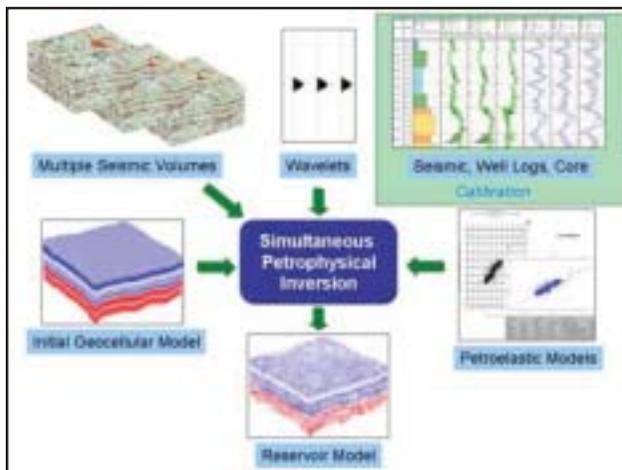
Fig. 1: Petrophysical Seismic Inversion workflow.
