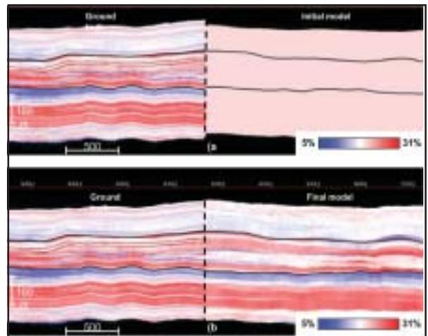
**Fig. 5:** Homogenous input cube of 20% porosity (top right) and “seismic-scale” result (lower right).
