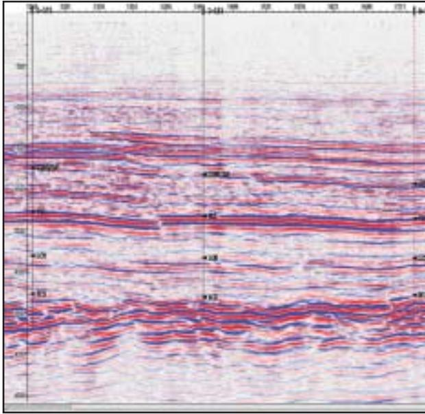
Fig. 7: Showing the well marker match with PSDM image.
