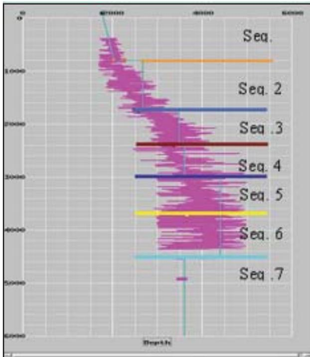
Fig. 2: showing the sequence boundaries along with sonic log and interval velocity model derived from seismic data. Note the match of seismic derived gradient to sonic gradient in the first sequence.
