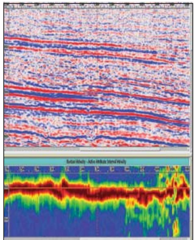
Fig. 3: showing the dependence of interval velocity on structural trend. Note the increase in interval velocity with depth.
