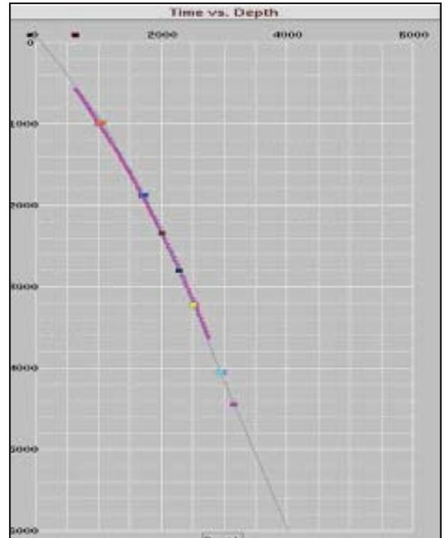
Fig. 9: Showing the match between the VSP time-depth curve and time depth curve derived from interval velocity volume. (Note the very good match between the two)
