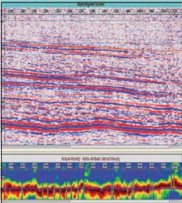
Fig. 5: Showing that velocity is not following structural trend for this sequence
