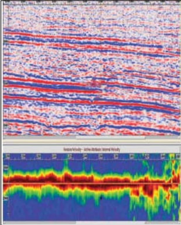
Fig. 4: Showing the removal of compaction effect by using a gradient value  $0.3 \text{ sec}^{-1}$
