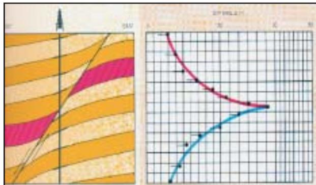
**Fig.1:** Ideal dip characteristic pattern for normal drag fault
