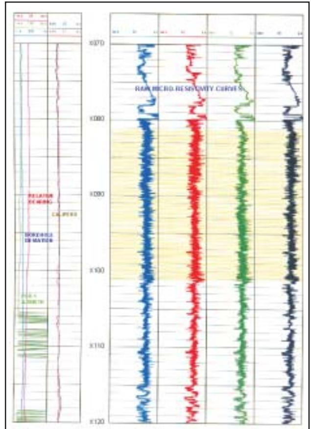
Fig.3: Raw microresistivity and auxiliary curves of dipmeter log of Baramura-A. Deformed zone is indicated by shaded portion.
