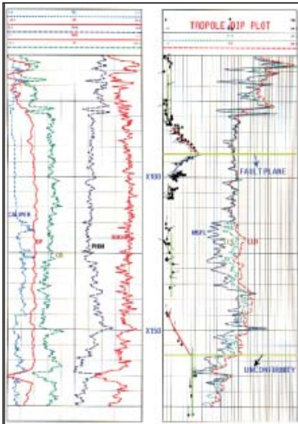
Fig.2: Dip arrow plot along with correlation logs in the interval X060-X180m of well Baramura-A
