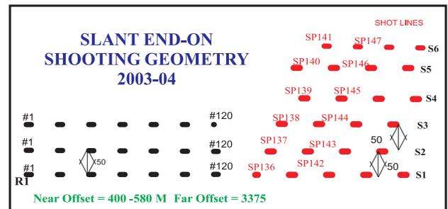
Fig. 3: Acquisition Geometry for the Slant End-on shooting
