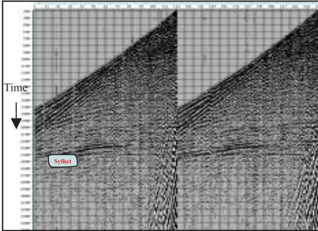
Fig. 9: A raw records from 3D data volume acquired using Slant geometry
