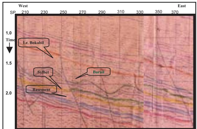
Fig. 13 : Interpreted 2D seismic section
