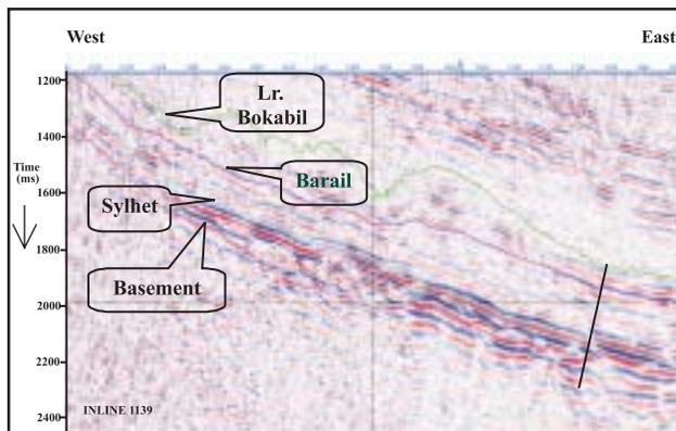
**Fig. 14 :** Interpreted Seismic Section From 3D data volume acquired using Slant End-on shooting geometry
