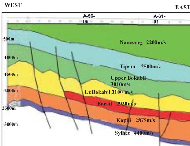
Fig. 2: Seismo-Geological Cross Section
