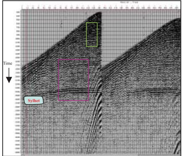
Fig. 11 :A Raw Records from 3D data volume acquired using Orthogonal geometry
