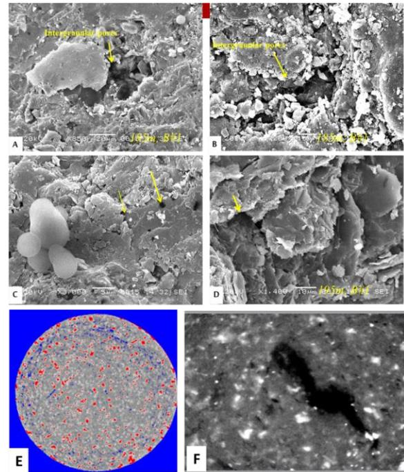
Fig 2. Photomicrographs. A. Intergranular pores in Raniganj shale, B. Intergranular shale in Cambay shale, C. Intragranular and matrix pores in Barren Measures shale, D. pores between the grains and matrix, E. m CT image showing fracture porosity, F. m CT image showing pores associated with organic matter.
