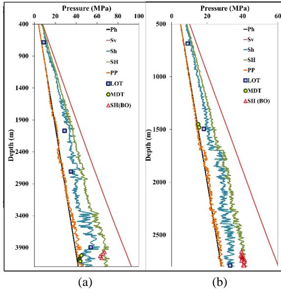
Figure 2: (a) and (b) hydrostatic stress ( $P_h$ ), vertical stress ( $S_v$ ), minimum ( $S_h$ ) and maximum ( $S_H$ ) horizontal stress, pore pressure (PP), leak off test data (LOT), modular tester data (MDT), and breakout derived maximum horizontal stress ( $S_H(BO)$ ) have been plotted against depth for wells M1 and M3.
