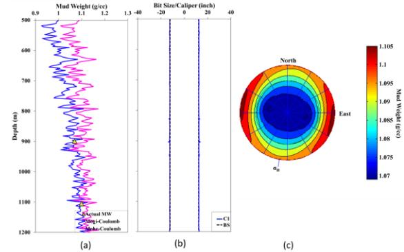
**Figure 4:** (a) Minimum MW for MG and MC derived rock failure criteria along with actual MW used while drilling well M3 for interval 500-1200m (b) Bit/Size and Caliper against depth for the same interval. (c) Borehole collapse model at 899m displaying minimum MW required to prevent breakout using MG criteria. Colour bar shows required MW in specific gravity units. Direction of  $S_H$  has also been marked.
