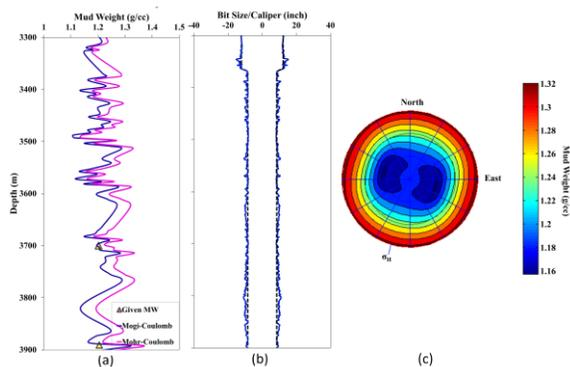
**Figure 3-** (a) Minimum MW for MG and MC derived rock failure criteria along with actual MW used while drilling well M1 for interval 3300-3900m (b) Bit/Size and Caliper against depth for the same interval. (c) Borehole collapse model at 3500m displaying minimum MW required to prevent breakout using MG criteria. Colour bar shows required MW in specific gravity units. Direction of  $S_H$  has also been marked
