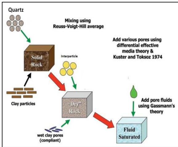
Figure 5: Schematic diagram of Xu – White RPM.
