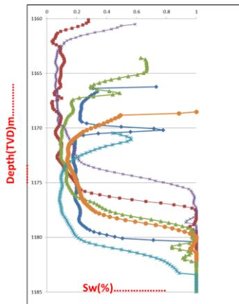
Fig.4 Saturation height function of initial wells of KS-VI sand
