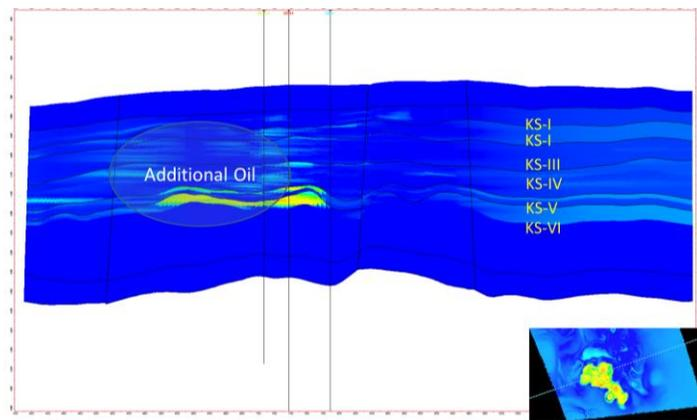
Fig.11 E-W cross sectional view depicting additional oil volume for KS-VI sand.
