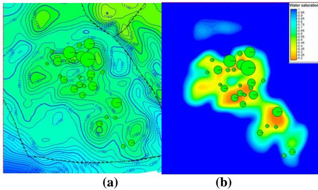
Fig. 9a Structure map on top of KS-VI reservoir 9b. Average saturation map of KS-VI zone superimposed on production bubble map.
