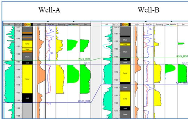
Fig.6 Generation of Sw log using saturation height function of KS-VI zone.
