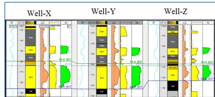
Fig.8 Generation of Sw log in old wells using saturation height function of KS-VI zone.
