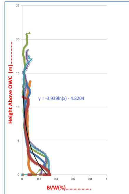
Fig.5 Saturation height function initial wells of KS-VI sand taking depth against BVW( product of porosity & saturation)
