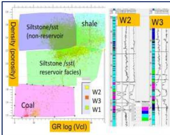
**Figure 11:** Crossplot of Gamma Ray log (Vcl) and Density (porosity) for rock physics classification and creation of litholog
