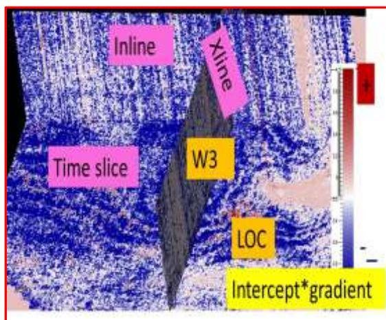
**Figure 15: Inline, crossline and time slice extracted from AVO Attribute volume showing class 2p effect near new location**
