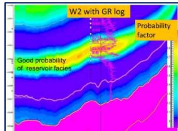
**Figure 13:** Probability factor analysis for reservoir facies and vertical section of litho-probability extracted from volume
