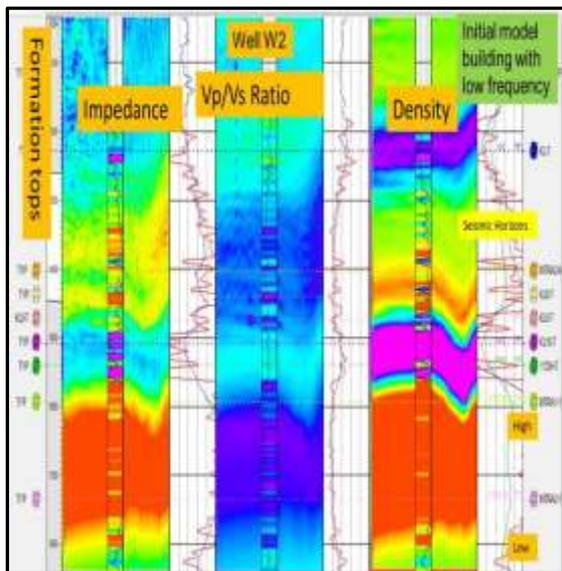
**Figure 5:** P wave impedance, Vp/Vs ratio and density inversion model result showing good match between log derived values and inversion results
