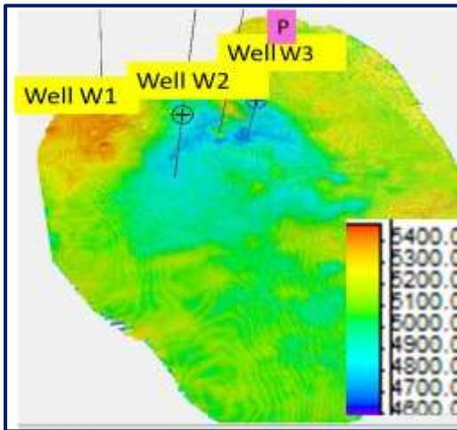
**Figure 9:** Acoustic impedance map at reservoir layer within Kalol formation
