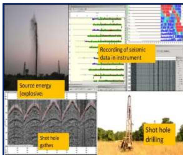
**Figure 1:** Seismic data acquisition and quality control during parameter fixation and experimentation
