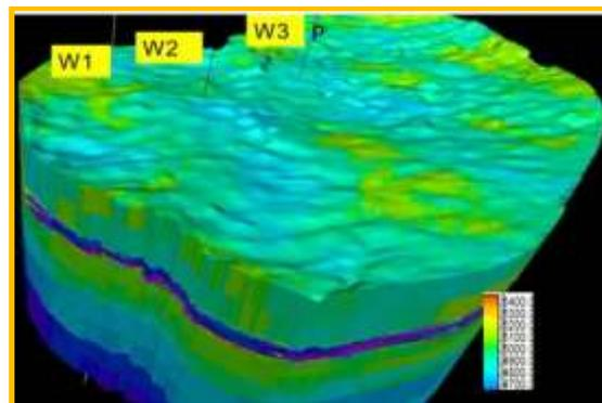
**Figure 7:** Acoustic impedance volume computed from 3D seismic volume
