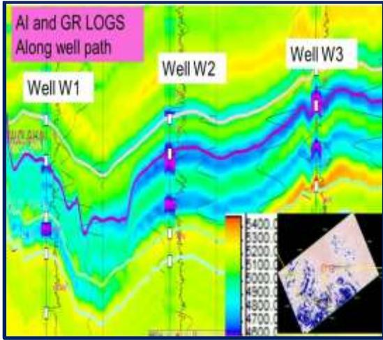
**Figure 8:** Vertical section (arbitrary line) extracted from acoustic impedance volume and passing through wells.
