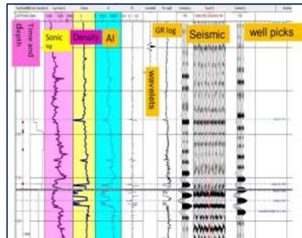
**Figure 4:** Synthetic seismogram showing correlation and well to seismic tie
