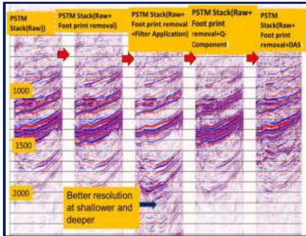
**Figure 2:** Seismic data processing and parameter fixation
