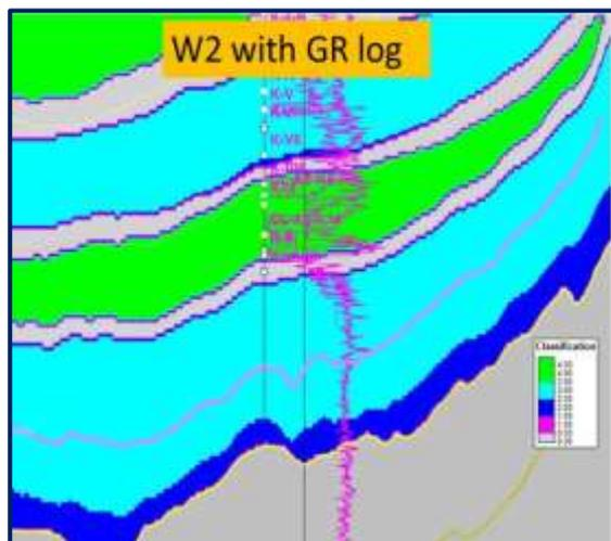
**Figure 12:** Rock facies classification based on xplot. Four classes as reservoir siltstone/ sandstone (green), shale (light blue), coal (light pink) and non-reservoir sandstone/siltstone (dark blue)
