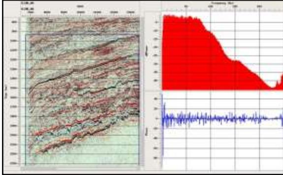
Figure 1: Spectrum of Broad Band Seismic Data (Peak frequency 24 Hz, Bandwidth: 2.5-90 Hz at -12 dB).
