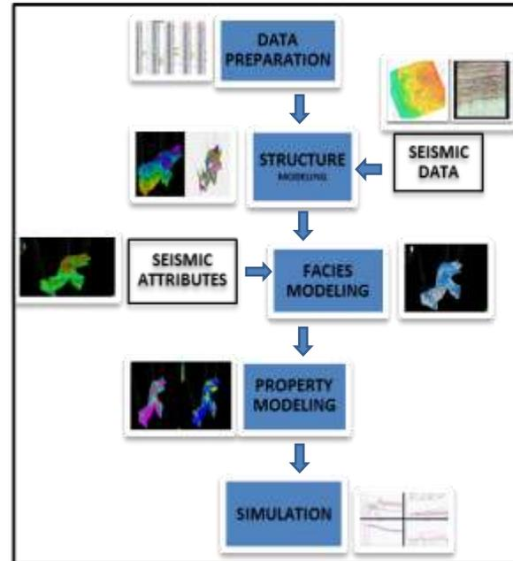
Figure 2: Workflow for building an integrated 3D static model
