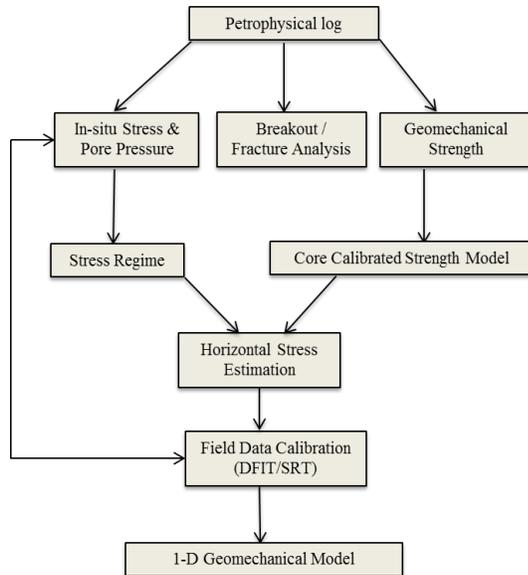
Figure 3: Workflow for 1D-Geomechanical Model
