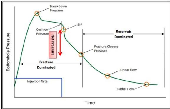
Figure 8: Cartoon illustrating CP, ISIP & NP from an injection fall-off test
