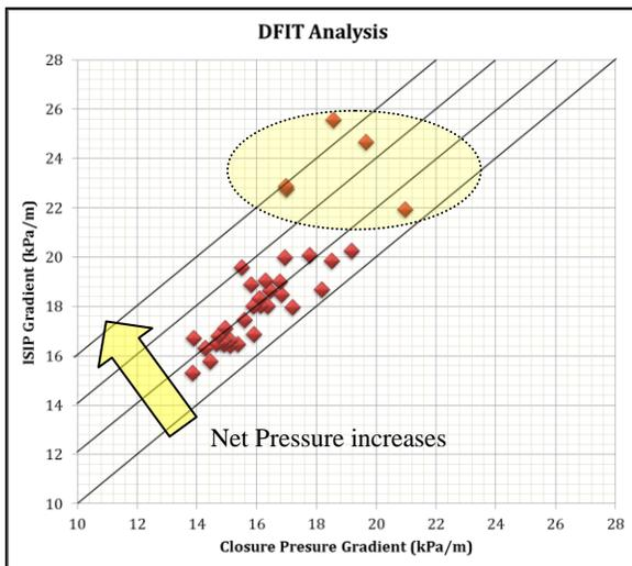
Figure 9: CP and ISIP plot from DFIT showing area of increasing net pressure and highlighted region where frac issues were encountered
