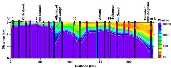
**Figure 3:** Subsurface electrical resistivity section obtained by Occam inversion of MT data. Locations of major rivers and cities are also marked.
