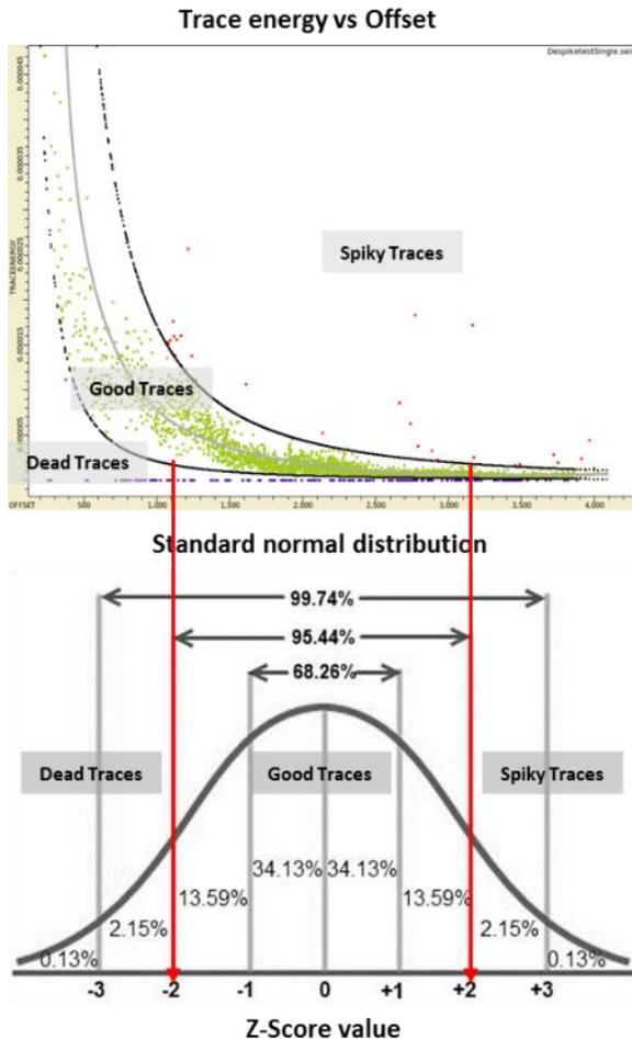
Figure 2: Trace classification using curve fitting
