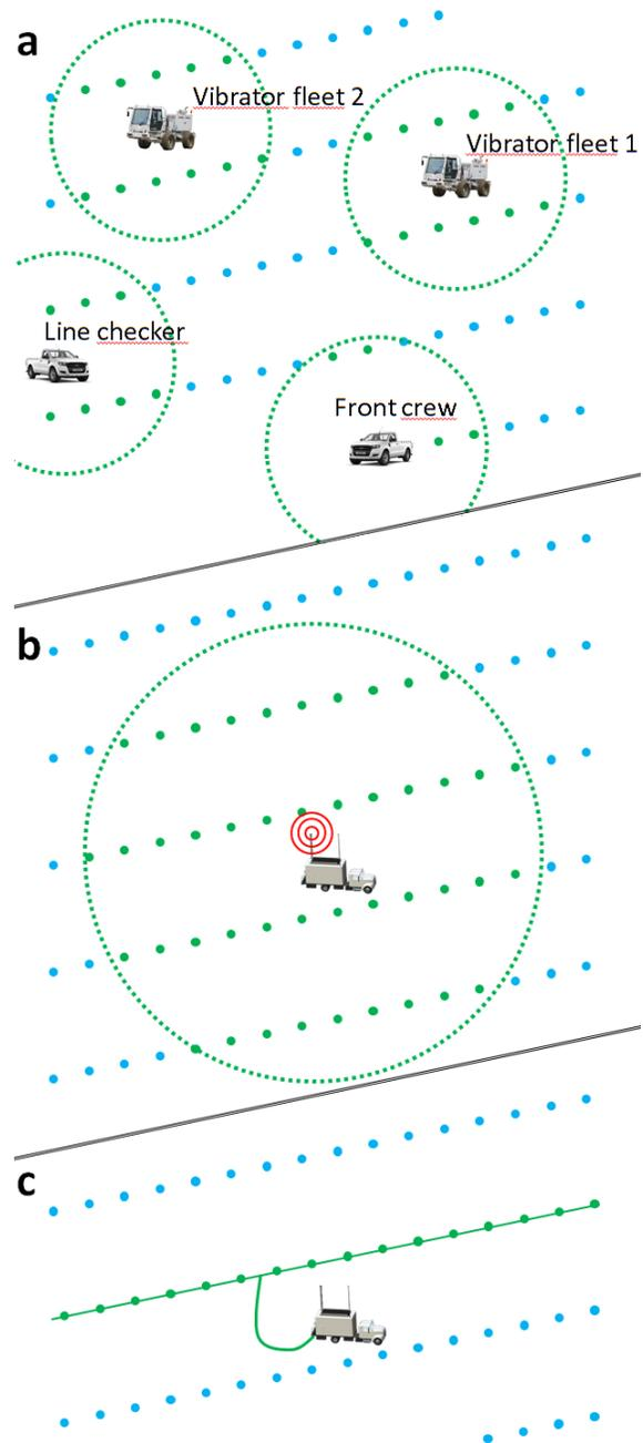
Figure 3: (a) opportunistic harvesting, (b) equipment and seismic data QC around recorder. Extra antennas (not represented) can be installed. (c) a wireless spread complemented by a cabled line. Channels harvested are displayed in green. For (b) and (c), data and QC are available in real-time. Note that spread proportions and distances are not respected.
