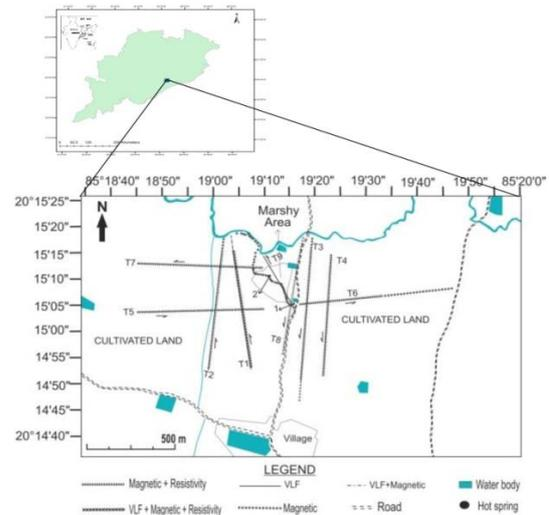
Figure 1: Map showing the geophysical survey profiles in Tarabalo Hot Spring Area
