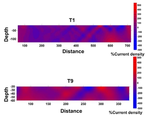
Figure 3: Current density cross-section of VLF profiles along T1 and T9 in Tarabalo region.
