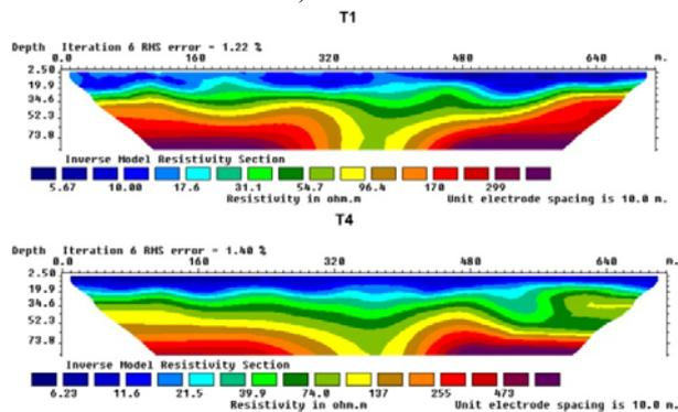
Figure 2: Apparent resistivity cross-section along profiles T1 and T4 in Tarabalo region.
