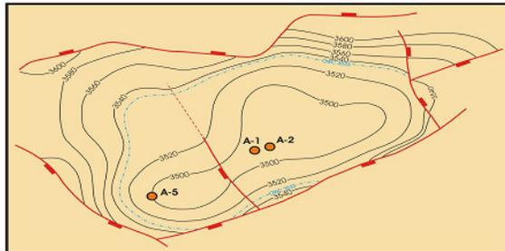
Fig.1: Structure contour map at top of Unit-II
