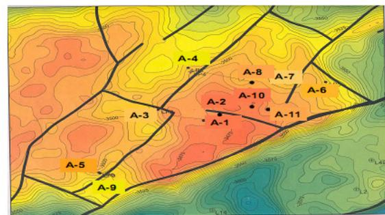
Fig.3: Revised structure contour map at top of Unit-II
