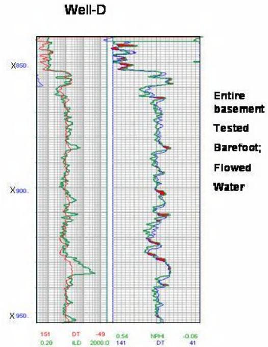
Figure-4. : Example of a dry well where no separation on log overlays
