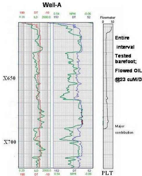
Figure-1: Example showing positive separation indicating hydrocarbon bearing zones
