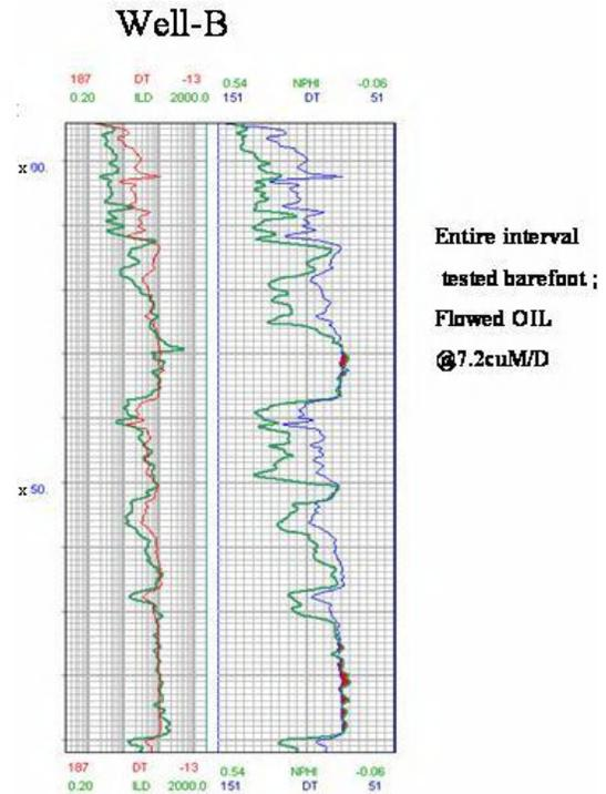
Figure-2: Example showing positive separation indicating hydrocarbon bearing zones.
