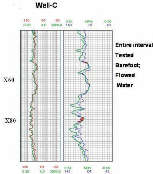
Figure-3: Example of a dry well where no separation on log overlays.
