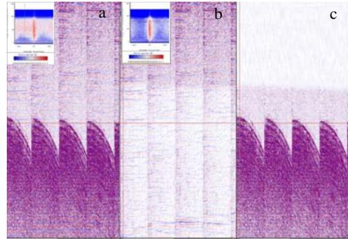
Figure14: (a) CDP gathers before High resolution Radon, (b) CDP gathers after High Resolution Radon and (c) Difference
