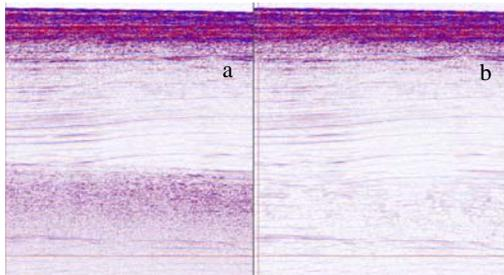
Figure 15: Stack sections (a) before and (b) after diffracted multiple attenuation.
