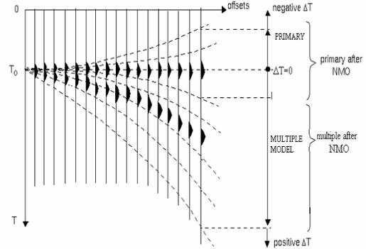
Figure 13: The RADON parameter definitions.
