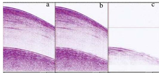
Figure 7: (a) SP before 2DSRME, (b) SP after 2DSRME; and (c) Difference
