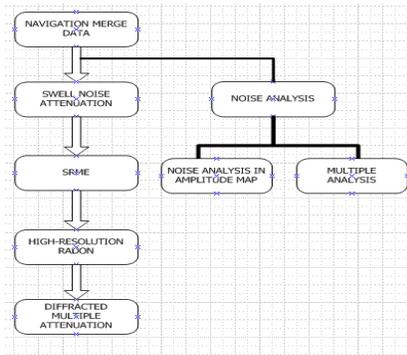
Figure 1: Flow Diagram of basic steps used for noise and multiple attenuation.
