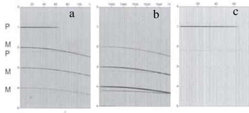
Figure 6: (a) Input data, (b) Multiple Model and (c) Adaptive subtraction
