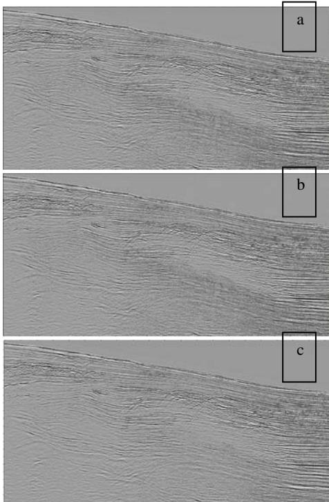
Figure 12: (a) Input stack, (b) 2D SRME output (c) Advanced 3D SRME.
