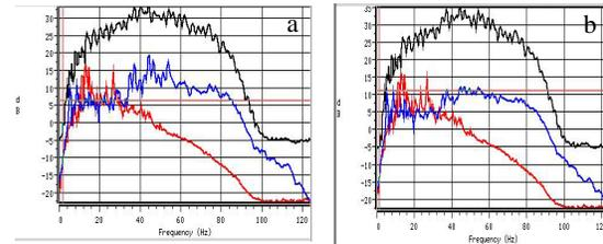
Figure 9: Frequency spectrum (a) before and (b) after 2D SRME at three different depth levels. Black represents shallower section, red represents above multiple zone and blue represents within multiple zone.
