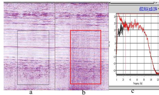
Figure 5: (a) Stack before swell noise attenuation, (b) Stack after swell noise attenuation and (c) Spectral analysis
