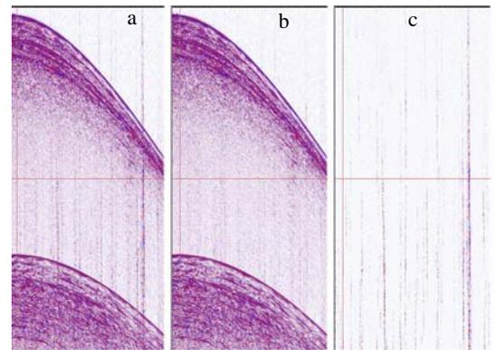
Figure 4: (a) Input SP for swell, (b) SP after swell noise attenuation and (c) Difference section.
